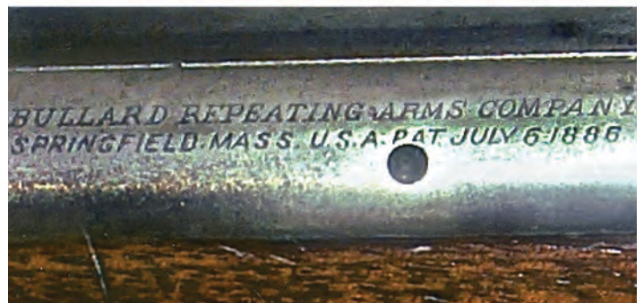
Extractor removal access hole location
