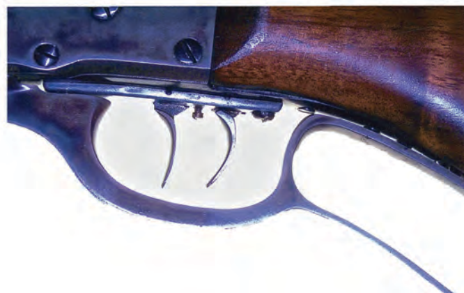
Cheek Piece (Top) and Schuetzen Detachable Triggers (Above).
