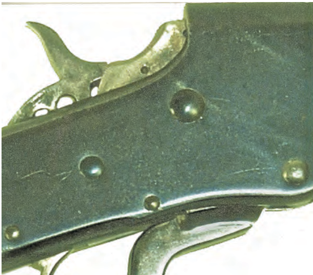
Sr. No. 3527 with Experimental holes to lighten weight of hammer.
