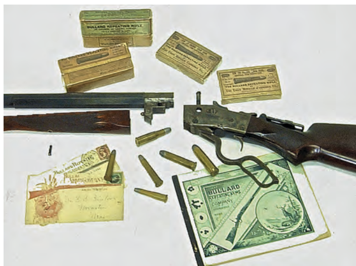
Detachable-Interchangeable Barrel Rifle taken apart.
