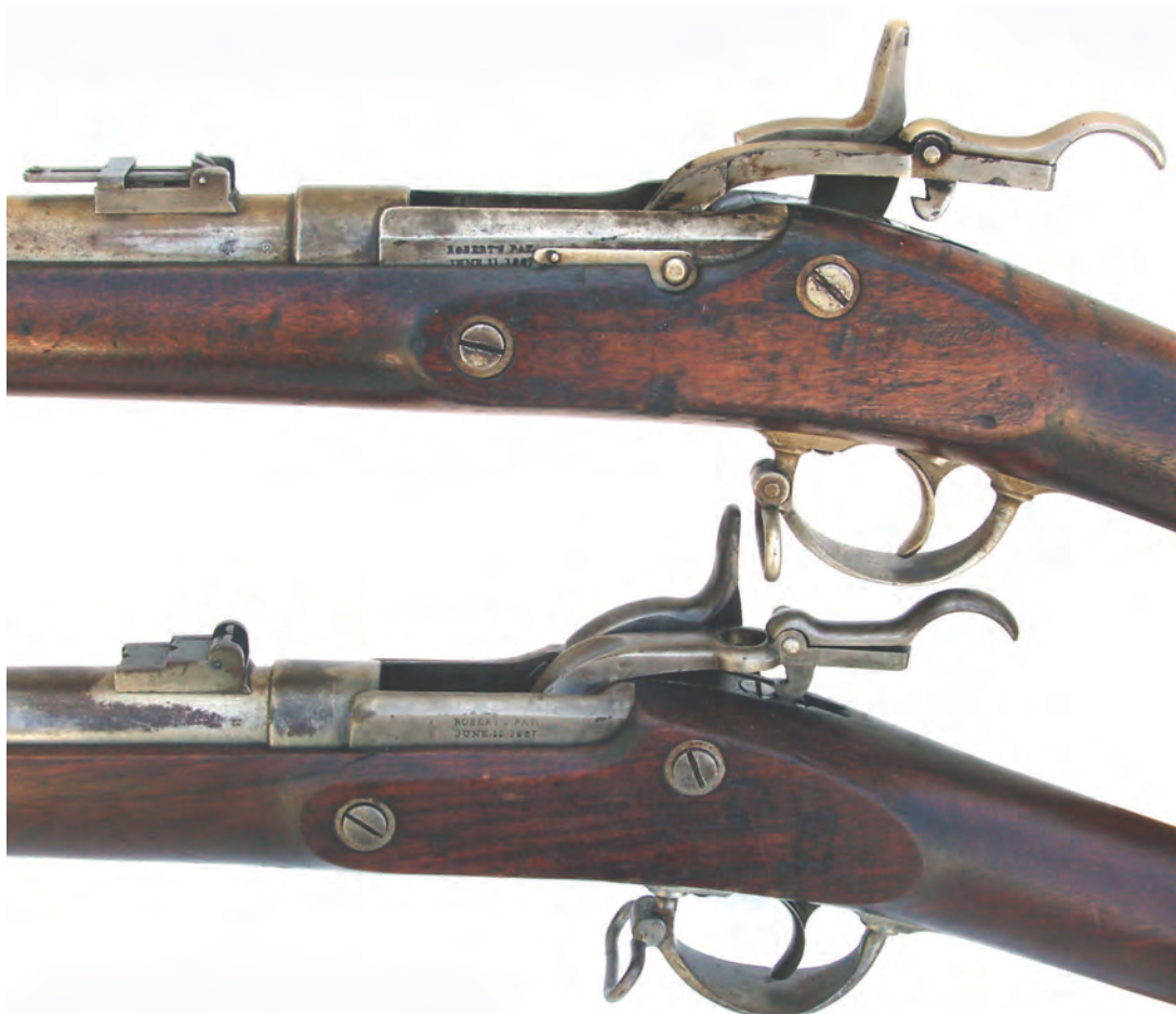
Plate 10. Comparison of the Short Frame (bottom) and Long Frame (top) breeches. The frames differ by one inch in length. (Author's collection and photograph)
