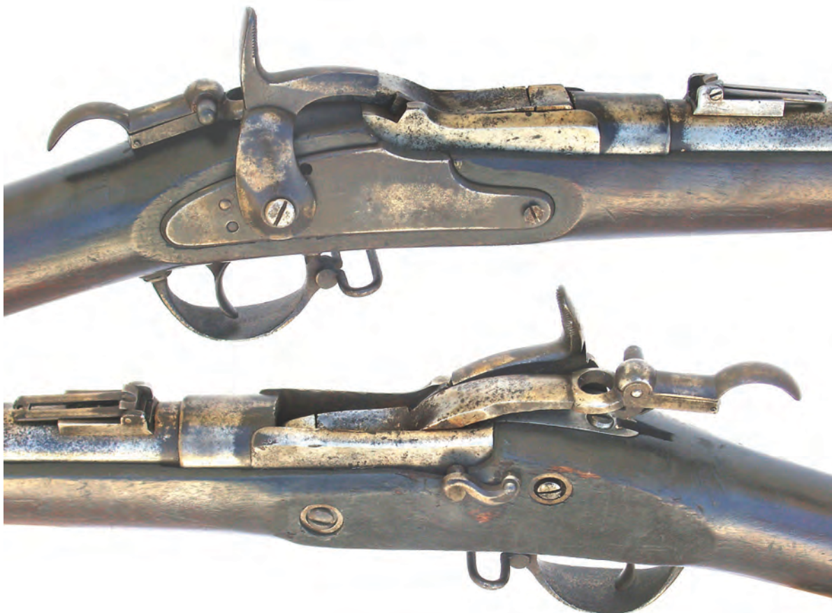
Plate 14. Transition model Roberts Long Frame example, handmade for the 1867 New York States Ordnance Board. The frame is 4-5/16 inches long. The breechblock is retained by a screw-in pin. (Author's collection and photograph)
