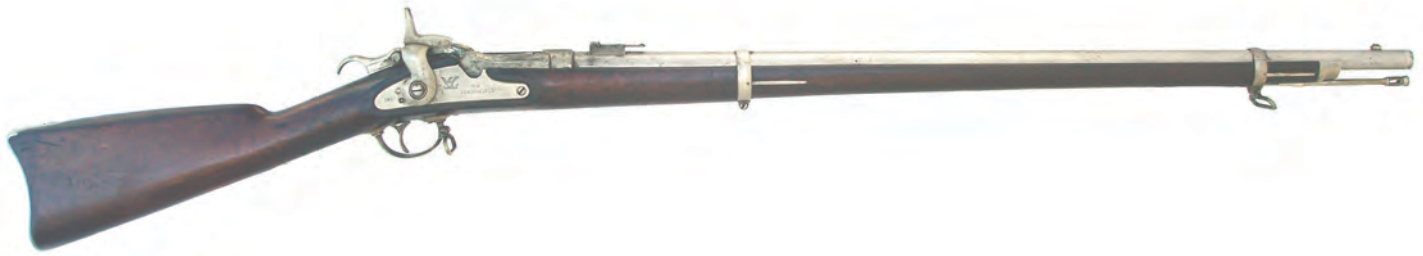
Plate 18. This fully tinned Roberts Long Frame rifle in caliber .50-70 has a barrel 32-1/2 inches long. Overall it emulates the Springfield Model 1868 rifle. Serial numbered “2,” this is likely Roberts gun #2 of the U.S. Navy trials. (Author’s collection and photograph)
