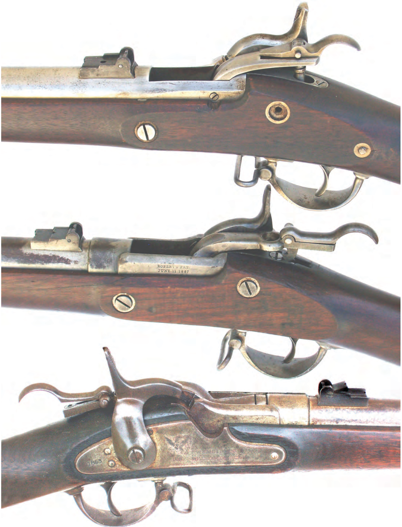
Plate 4. Comparison of the 1866 prototype (top) and a production Short Frame type (center & bottom), showing the incorporation of a frame for the breech. The frame is 3-1/2 inches long, not including the tang. (Author's collection and photograph)
