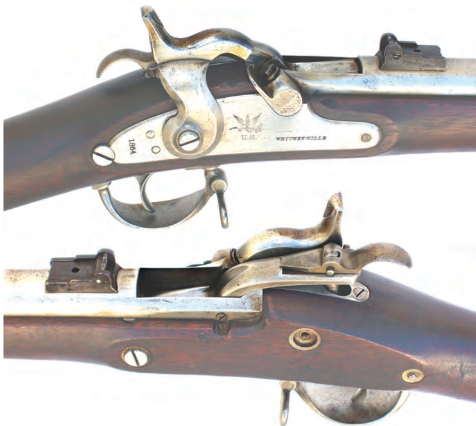
Plate 3. Prototype Roberts breechloader made for the 1866 Ordnance Board. The breechblock is set directly into a slot in the barrel. (Author's collection and photograph)
