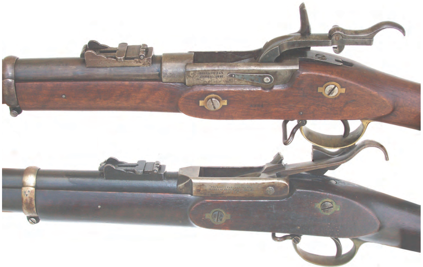
Plate 13. Comparison of the Roberts Long Frame (top) and Peabody Patent (bottom) breeches. Both are .58 caliber centerfire. (Author's collection and photograph)
