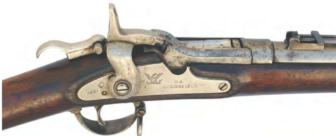
Plate 9. A close-up of the breech of another Long Frame type. Note the bolt which replaces the front lockplate screw and is screwed into the frame. The frame is 4-1/2 inches long, not including the tang. (Author’s collection and photograph)
