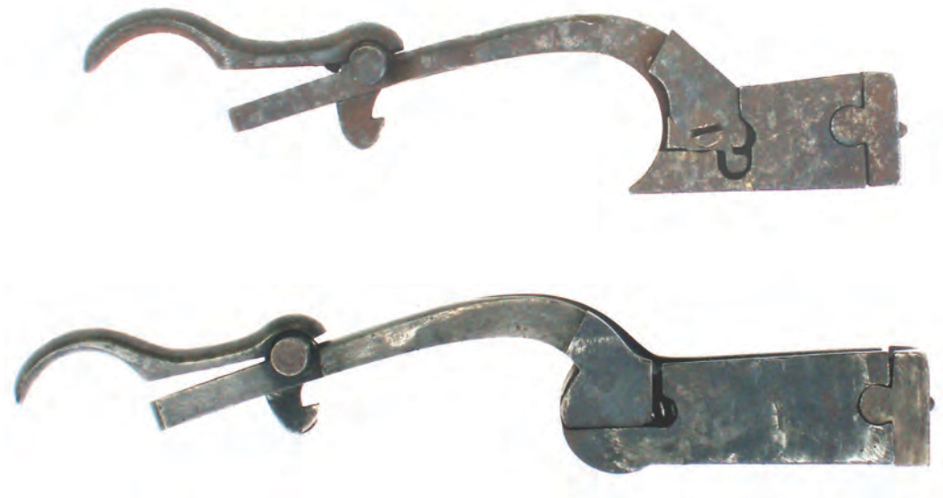
Plate 11. Comparison of the Short Frame (top) and Long Frame (bottom) breechblocks. (Author's collection and photograph)
