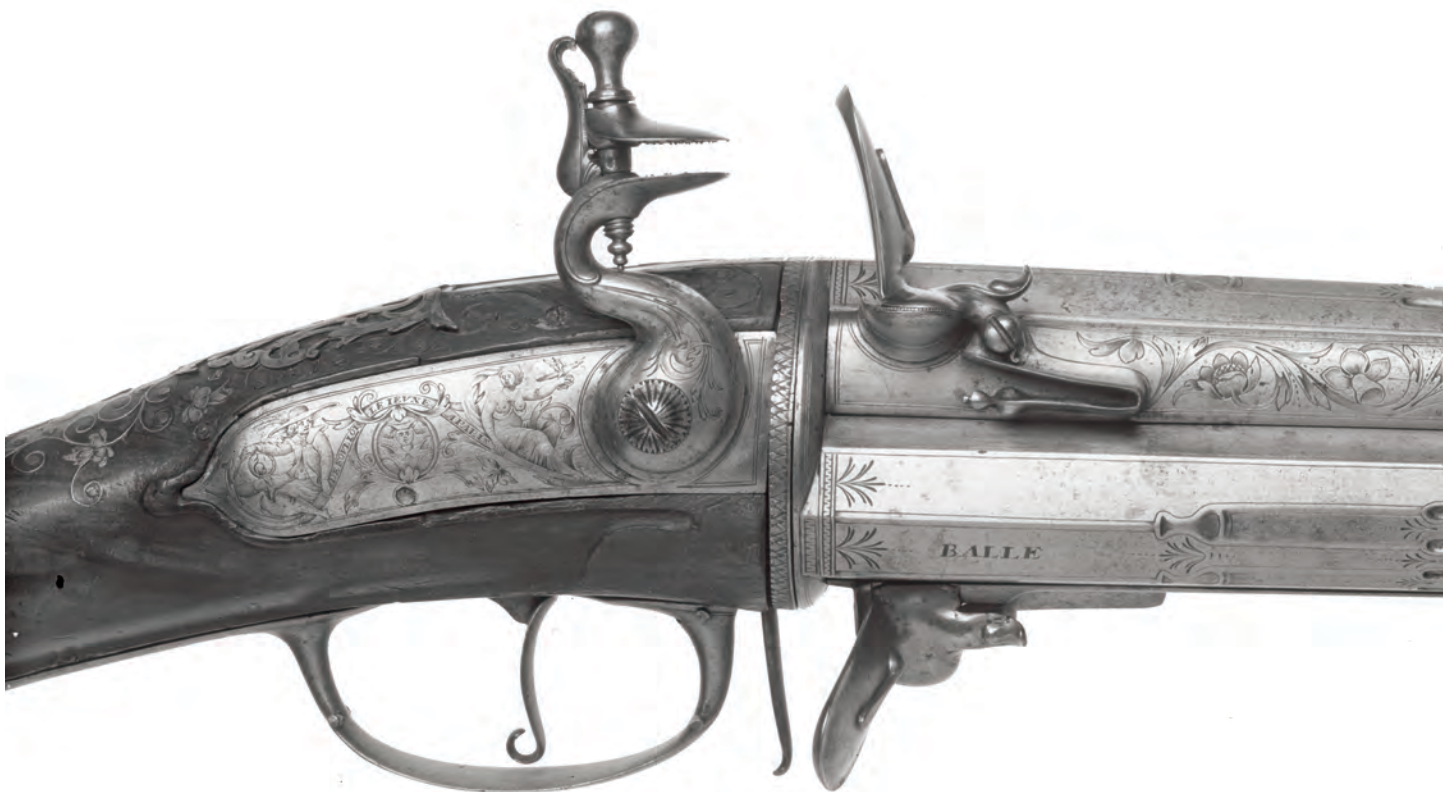
Fig. 9 Detail of the lock plate and revolving chambers of a revolving rifle signed DE FOVLLOIS LE JEVNE A PARIS in the collections of the Livrustkammaren, Stockholm, Sweden (Acc. No. LRK 3630 [old no. 1344]). Photograph courtesy of the Livrustkammaren.
