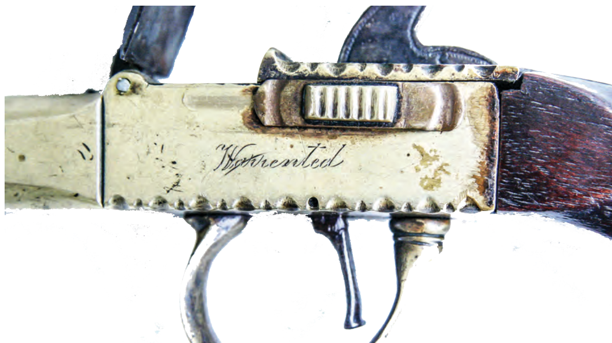
Figure 11. The reverse side of the breech area has just the word Warranted (sic) engraved on it. The sliding safety for the pistol is also on this side.
