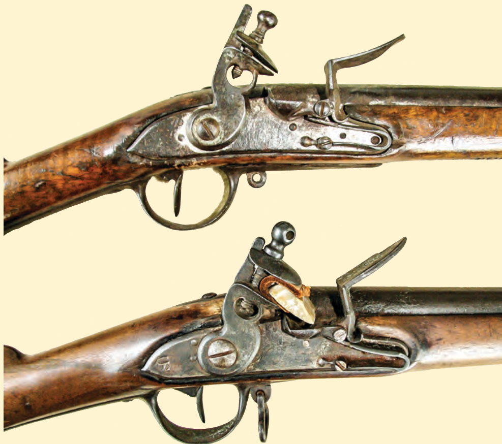
Figure 22. The lock areas of Haslett-marked muskets Nos. 1 (top) and 2 (bottom). The name of the original armory where the musket was assembled cannot be seen on the lock of No. 1; St. Etienne is on No. 2. Courtesy Helen and Edward Flanagan (top), and the author (bottom)
