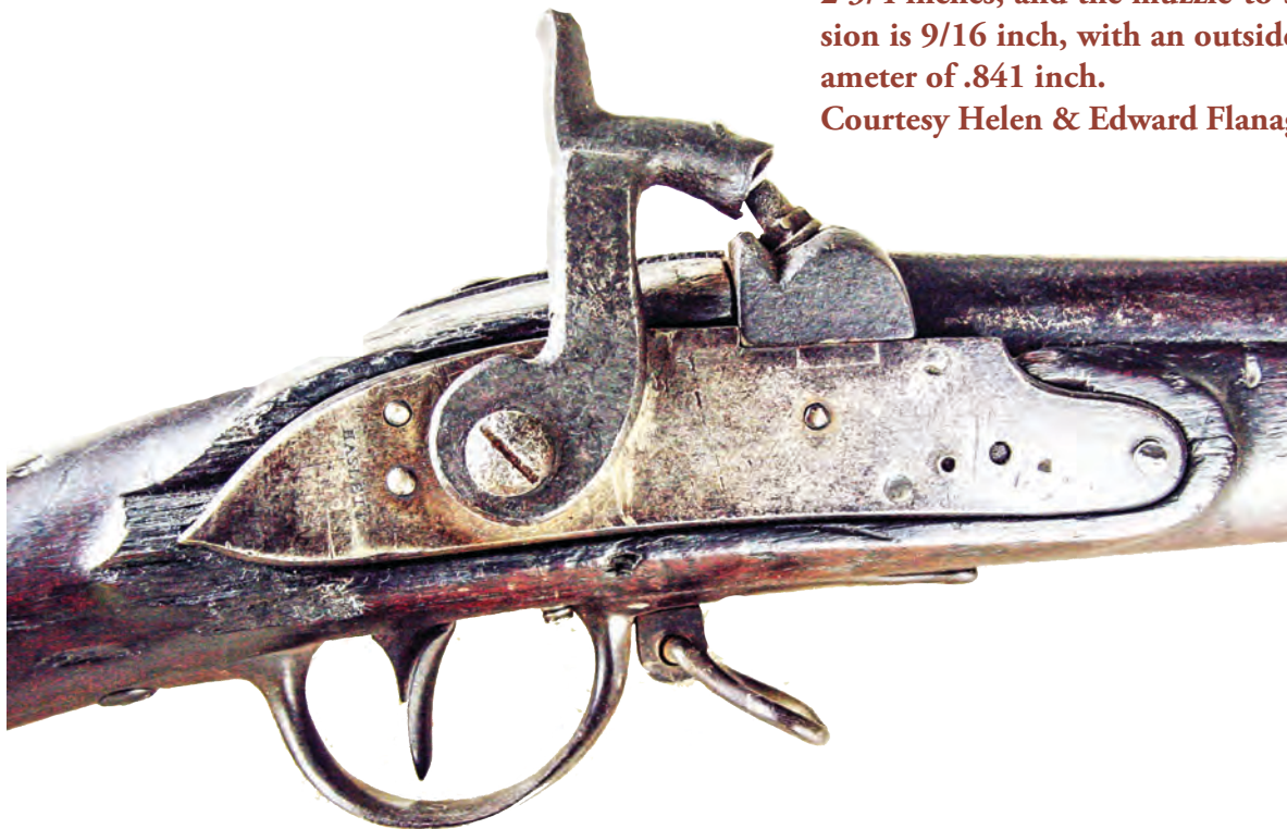
Figure 2. Lock of a musket manufactured by James Haslett for the state of Virginia, ca. 1801-2. The lock is simply marked HASLETT and the barrel is marked to Pittsylvania County. Based on the bolster used and how the pan area was filled in, this example was likely altered to percussion at the beginning of the Civil War by William B. and Cyrus Fisher in Lynchburg, Virginia. The hammer is a replacement for that used when the arm was altered to percussion. The muzzle extension is 2 3/4 inches, and the muzzle-to-stud dimension is 7/8 inch, with an outside muzzle diameter of .847 inch. Courtesy Helen & Edward Flanagan
