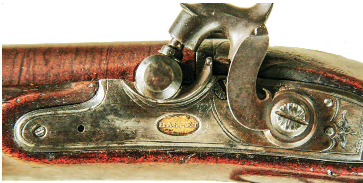
Figure 14. The left-hand lock of a double-barreled shotgun, altered to percussion, showing a typical inlaid gold planchett with HASLET (sic) stamped intaglio. An identical planchett, also misspelled, is on the right-hand lock. The alteration is well done, with metal finishing matching nicely. Since Haslett died just as percussion ignition systems were gaining acceptance in the United States, it is unlikely he made the alteration. Courtesy Helen & Edward Flanagan
