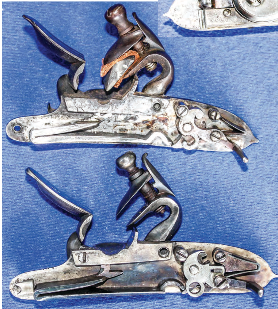
Figure 13, Interior view of Markley (Top) and Richards locks
