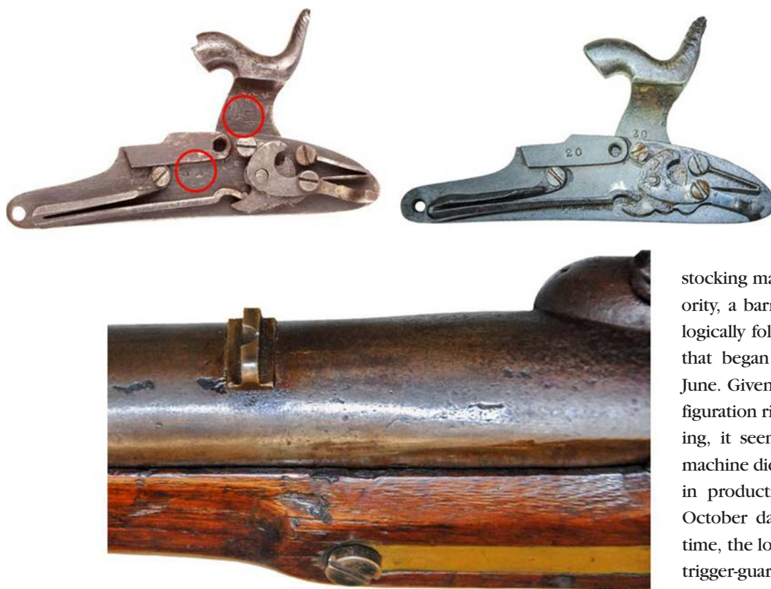
Figure 18. The locks of the late-production Wray collection rifle (LEFT) and the Winfield collection rifle (RIGHT) are marked on the inside of the hammers and on the inside faces of the lockplates with numbers “85” and “20,” respectively. The lock mechanisms are of generally good quality, albeit without mainspring swivels. Note the flaws on the surface of the wrought iron barrels, which were almost certainly made in Asheville.
