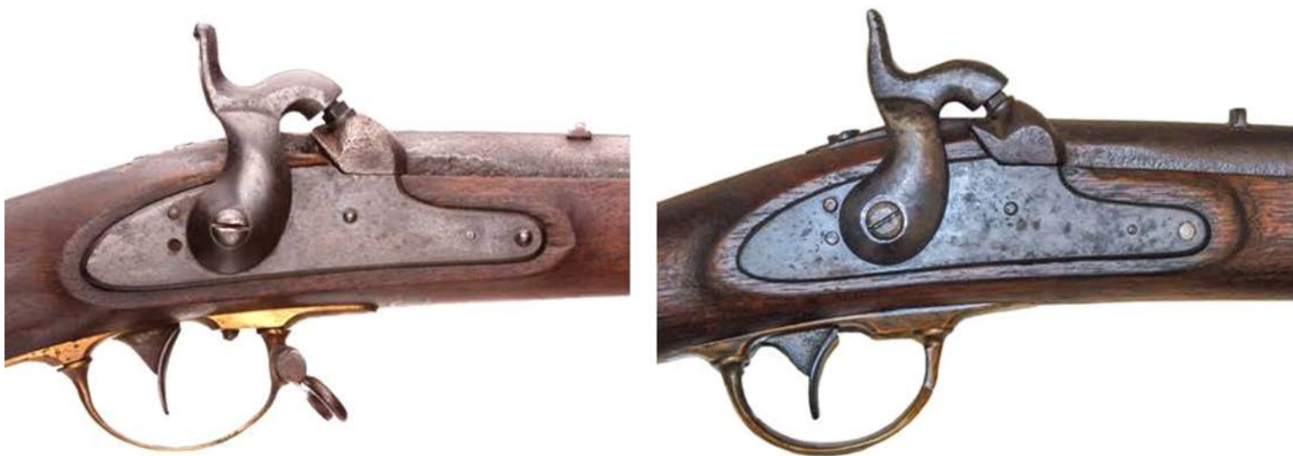
Figure 17. The features of second-configuration rifles are remarkably uniform, including (with a single exception) unmarked lockplates. Nevertheless, there are many small variations, such the addition of a re-used Model 1841 hammer (LEFT) on the DuBose collection rifle (“423”), and an unusually thick shield behind the cone seat (RIGHT) on the Winfield collection rifle (“x51”). Note also the lack of a rear sling swivel.
