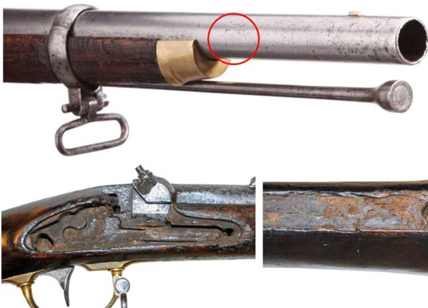
Figure 4. Numbered “116” under the barrel, this rifle from the Wray collection is believed to be one of the earliest ones fabricated at the Asheville Armory. Note the unusually thin barrel, a bayonet stud slot that may have been marked but never milled, and the obviously hand-bedded lock and trigger-guard cavities (with ramrod protruding into the lock cavity). Both bands are made of iron instead of brass and the forward one appears to have been taken from a British Pattern 1853 rifle-musket.
