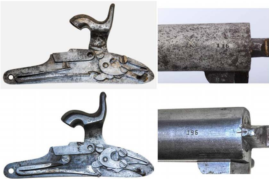
Figure 11. A comparison of the workmanship on rifles “116” (TOP) and “196” (BOTTOM) shows the considerably improved lock mechanism of the latter, including a mainspring swivel, a screw securing the upper mainspring branch, and a re-used Model 1841 hammer. Both locks were made under the supervision of Wesley Justus, who later claimed Union loyalties. The barrels of the two rifles are probably from the same source, though “196” is thicker-walled and better-finished. Both barrels are marked with the same set of dies.
