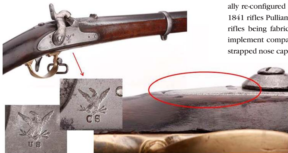
Figure 5. The first Asheville Armory rifles were assembled with re-used Harpers Ferry-made U.S. Model 1841 lockplates, the tails of which were ground off to obscure the markings. The original eagle stamp remains untouched but the “US” has been struck over to form “CS.”
