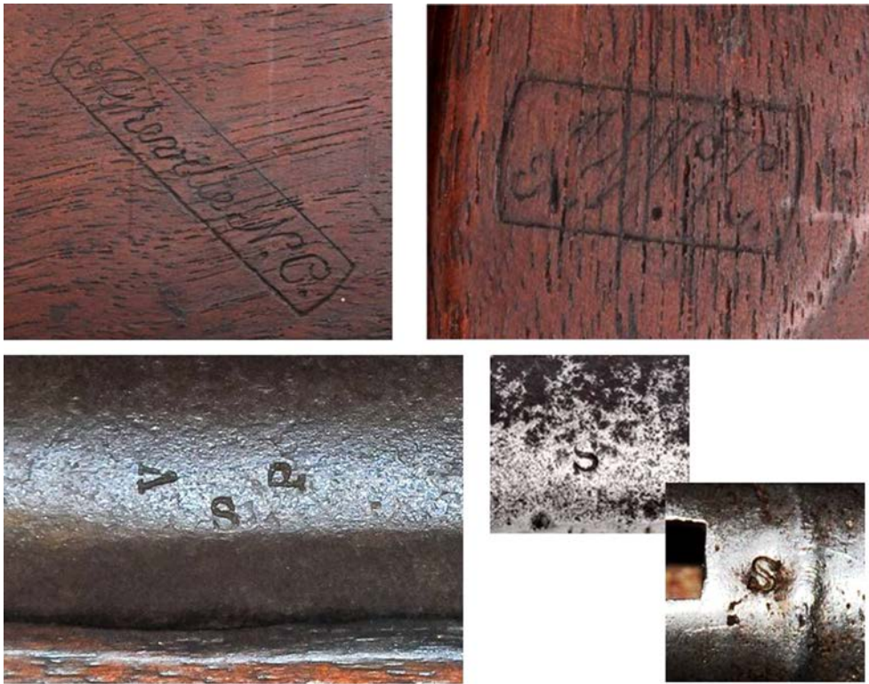
Figure 2. The rectangular inspection stamps “ASHEVILLE N.C.” and “A.W.K.” (for Master Armorer Amasa W. King) appear on stocks of both first and second configuration rifles. The “S” inspection stamp (believed to be for E.W. Stubbs, foreman of the barrel shop) appears most often on barrels of first configuration rifles. The “S” at lower right marks a socket bayonet made by the Union Manufacturing Company of Richmond. Could there be a connection between this “S” mark and the “S” on the barrels of Asheville Armory rifles?
