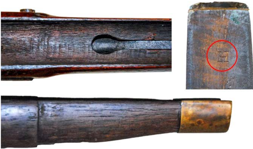
Figure 15. Evidence of machine-made stocks on second-configuration Asheville Armory rifles is clearly visible in the improperly-milled tip of the Albert collection rifle as well as the striations across the stock channel of the Wray collection rifle ("85") indicating use of a barrel-bedding machine. Note the stamped "H" assembly code on the butt of the DuBose collection rifle ("423").
