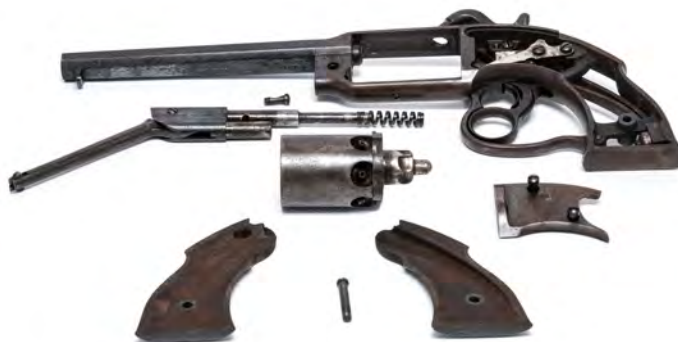
Fig. 39 - Savage Navy disassembled
