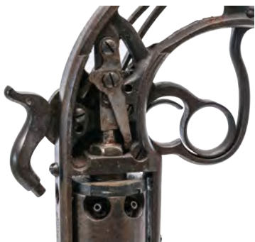
Fig. 40 - Savage Navy Revolver, toggle link starts to rise, the hand is down
