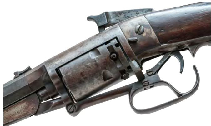
Fig. 8 - Lever partially opened, cylinder starts rotation
