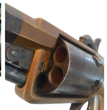
Fig. 14 - First Model Figure Eight variation with chamfered cylinder
