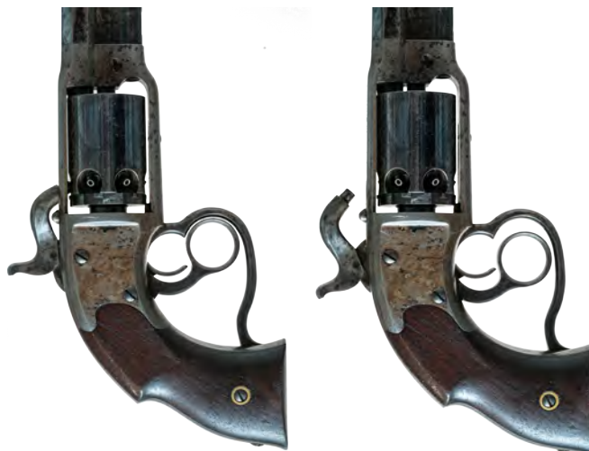
Fig. 35 - Hammer just off nipple
