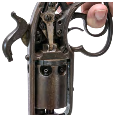
Fig. 42 - Toggle link is up and cylinder moves rearward.
