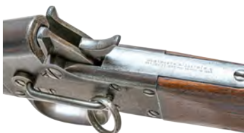
Fig. 58 - Hammer back, breech open, .46 Caliber Carbine
