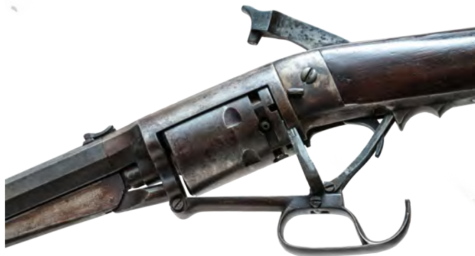
Fig. 9 - Lever down, cylinder rotated, fully cocked, cylinder wedge down
