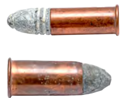
Fig. 55 - Comparison - .46 and .50 Caliber Cartridges
