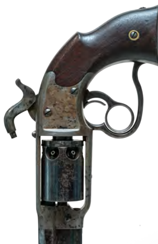
Fig. 43 - The revolver is at full cock, releasing the lower trigger allows the cylinder to move forward sealing against the barrel.
