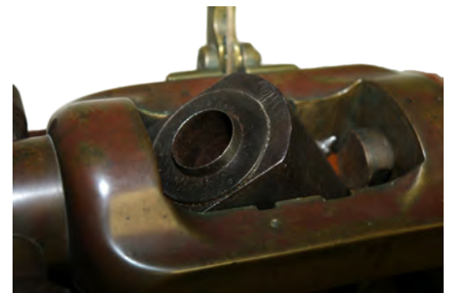
Figure 8 Comparison of tilted breech, breech seal and linkage, between patent drawing and Model Cannon. Note the similarities between the patent drawing and the model cannon in design and function.
