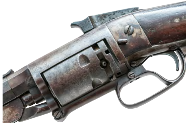
Fig. 7 - North and Skinner rifle with revolving breech (mfg. by North and Savage)
