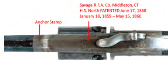
Fig. 31 - Anchor stamp on barrel, Savage Navy Revolver
