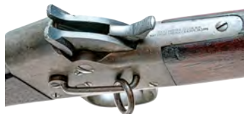
Fig. 60 - Hammer cocked Split Breech closed
