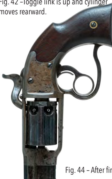
Fig. 43 - The revolver is at full cock, releasing the lower trigger allows the cylinder to move forward sealing against the barrel.
