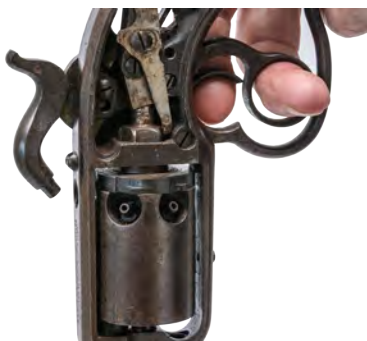
Fig. 41 - As trigger is pulled, the hammer lifts and the hand engages the ratchet
