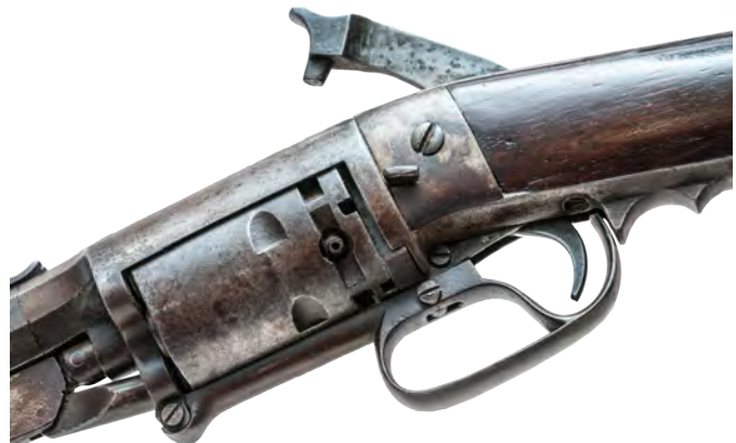
Fig. 10 - Lever up, wedge has pushed cylinder forward, ready to fire
