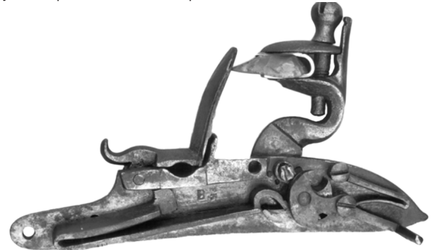
Figure 7 - Musket lock, Rappahannock Forge, Falmouth, Virginia; 1775-1781. Steel, iron. 1982-231 The Colonial Williamsburg Foundation, Museum Purchase. Note the "FK" initials on the lock plate, the mark of Frederick Klette. Joseph Perkin employed a similar style stamp with his own initials to mark locks made at Rappahannock Forge.
