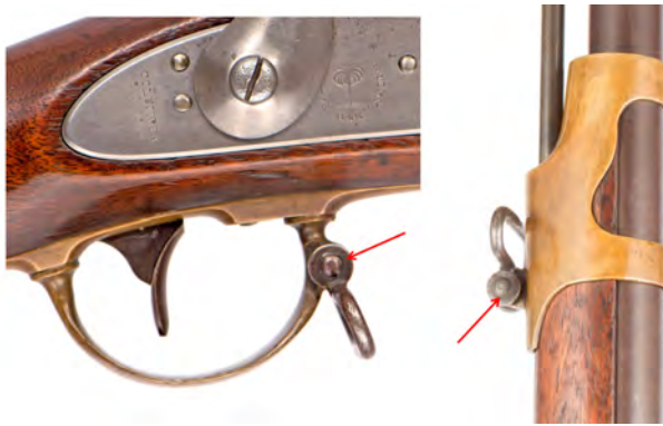
Figure 20 Note protruding rivets or pins of sling swivels on both the nose cap and trigger guard.
