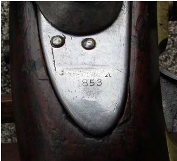
Figure 34. This FAKE Palmetto Rifle lock was a simplistic attempt to deceive using a scrubbed 1853 lock plate and adding the letters "C" - spaces - "A" above the 1853.
