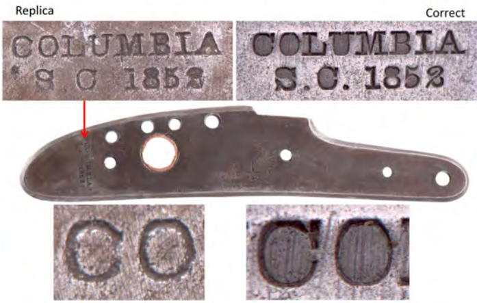
Figure 37. Note the Laser Cut Replica markings are very good facsimiles but careful examination shows the edges are not sharp. With a hand lens tiny individual laser hits or divots can be seen in the bottoms of the letters.
