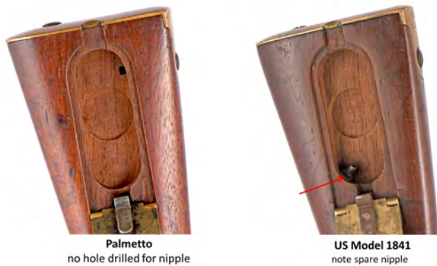
Figure 16. Note the US Model 1841 toolbox with spare nipple in place and the Palmetto Rifle toolbox without the hole for a spare nipple.
