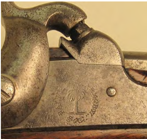
Figure 31. Apparently even a blurred double strike of the "Spiral Tree" Palmetto Armory insignia was not a sufficient cause for rejection of this pistol lock plate. COURTESY OF THE SMITHSONIAN INSTITUTE, WASHINGTON, DC.
