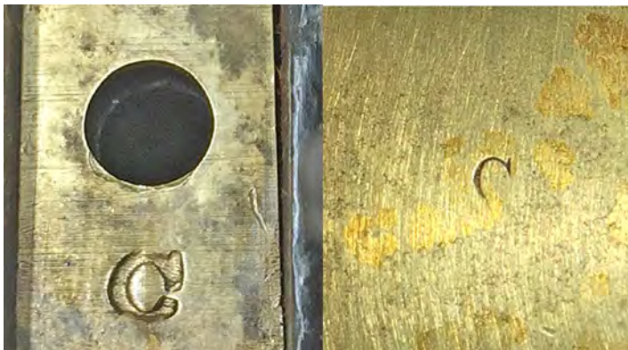
Figure 5 On the left is the large Condemnation "C" struck in a hidden location, in this case the backstrap of an 1842 pistol. On the right is a small fine Federal Inspector initial "c". In this case, the "c" was struck on the exposed surface of a Robbins & Lawrence 1841 rifle trigger bow.
