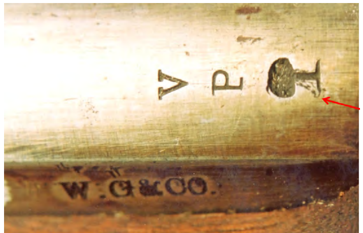
Figure 3. This photo shows a Palmetto Musket barrel retaining Springfield "VP Eagle" proof marks. - Courtesy of the Virginia Historical Society (#990.100.125).
