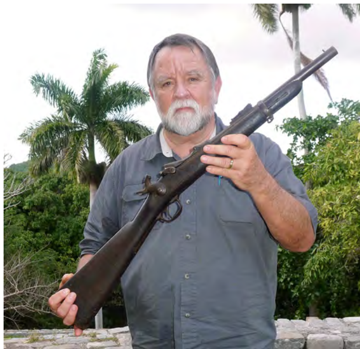
Steve Helsley holds Ernest Hemingway's Springfield Model 1873, Serial No. 13591—originally a trapdoor cavalry carbine (note the saddle-ring swivel bar). Despite its Custer Range number, this is one of a relative handful of trapdoor rifles that was shortened and bored out by the Springfield Armory to serve as line-throwing and harpoon guns. Hemingway bought it from Abercrombie & Fitch in November 1928 for $60. (Steve Helsley)
