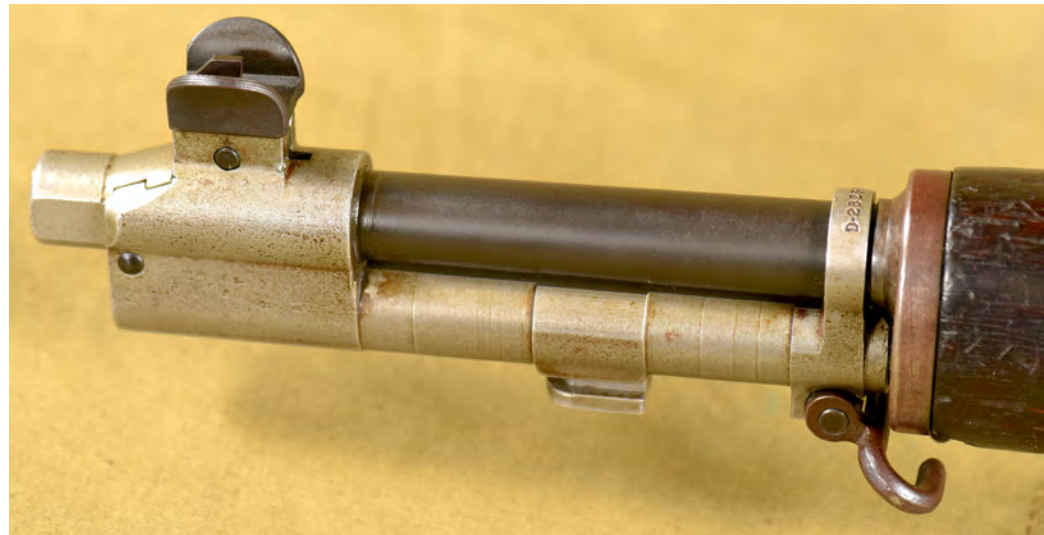
Figure 2. First design Type 2 "Gas Trap M1 Garand" screw-on type gas cylinder.
