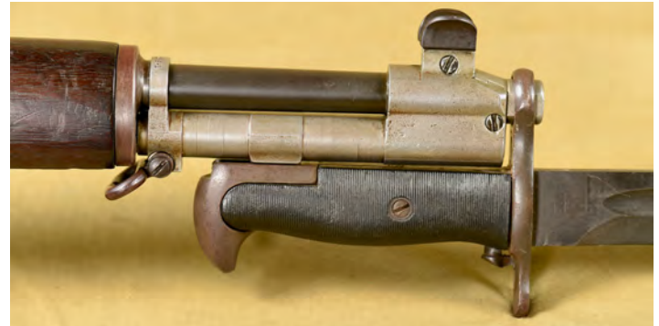
Figure 6. The first design screw-on "Gas Trap" gas cylinder was thought to be too weak to support the bayonet during combat use.
