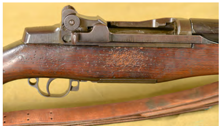
Figure 10. Dents in the right side of the stock were caused striking the points of the .30-06 cartridges in 8-round enbloc clips against the stock to ensure that the cartridges were completely seated in the clip.
