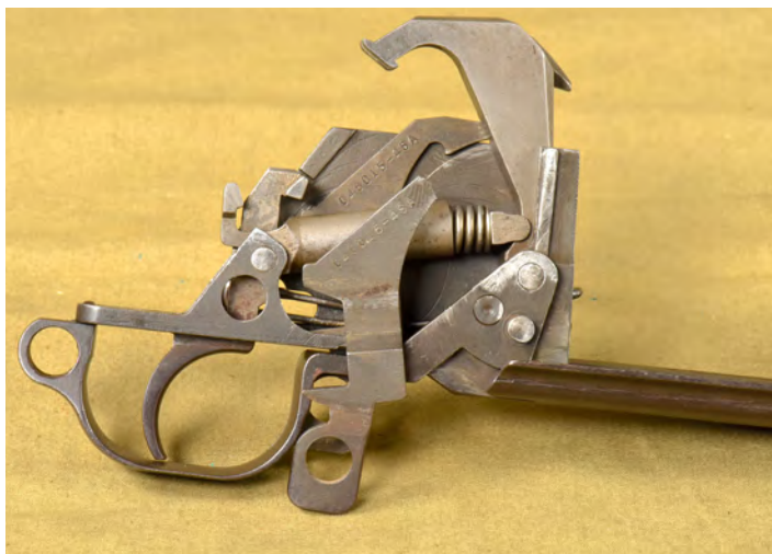
Figure 12 Photo shows the original modified safety with the tip broken off (in front) compared to an installed replacement unmodified safety. The modification was done in the field to make the safety quieter to engage and disengage.
