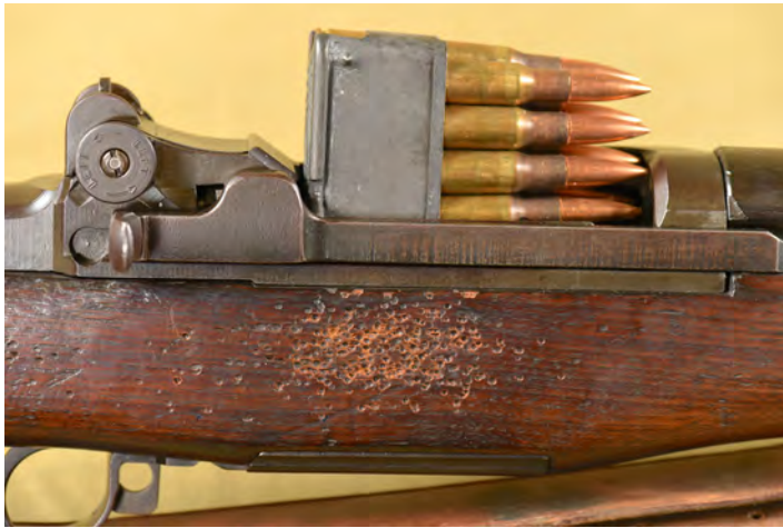
Figure 11 If the cartridges in the 8-round enbloc clip are not completely seated in the clip, it is difficult, if not impossible, to load the rifle.
