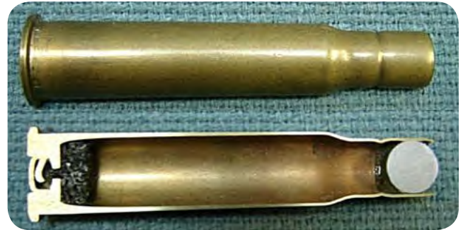
Fig. 22 - .30 caliber gallery practice cartridge for Krag rifles and carbines with round ball and smokeless powder.
