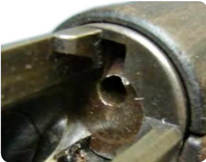
Fig. 32 - Breech of Stevens-Pope .22 caliber Krag showing use of standard extractor.
