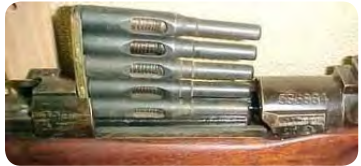
Fig. 34 - Model 1903 .22 Gallery Practice Rifle ("Hoffer-Thompson") showing the cartridge holders with .22 short cartridges being loaded into the magazine, the same as if it were the .30 caliber rifle.
