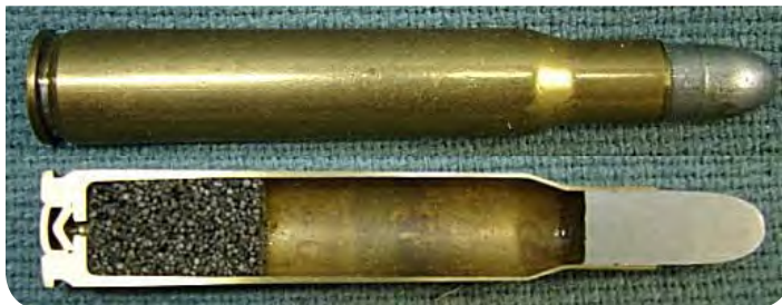
Fig. 27 - Caliber .20 Gallery Practice Cartridge Model of 1919, sectioned.
