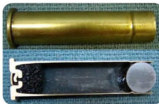
Fig. 17 - Gallery practice cartridge for .45-70 rifles or carbines with round ball and 5 grains black powder.
