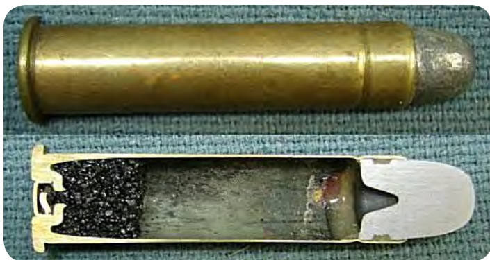
Fig. 21 - Gallery practice cartridge for .45-70 rifles or carbines with 230 grain conical bullet.
