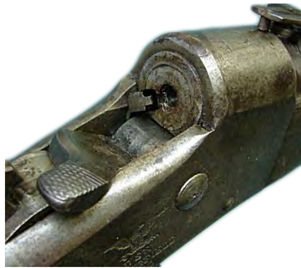
Fig. 31 - U.S. Navy Model 1870 .50-70 rifle converted to .22 rimfire in 1889 by Winchester.
