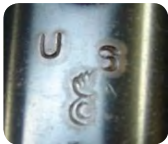
Fig. 37 - The Winchester gallery practice rifles purchased for military use were marked with hand stamped U.S. and ordnance bomb, however they are easily faked.
