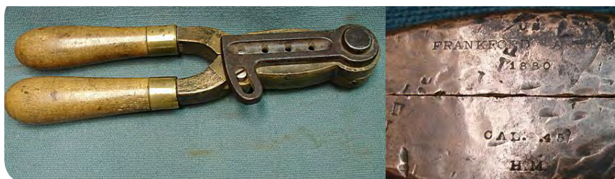
Fig. 18 - Frankford Arsenal .45 caliber round ball mold for local use casting gallery practice bullets, dated 1880.
