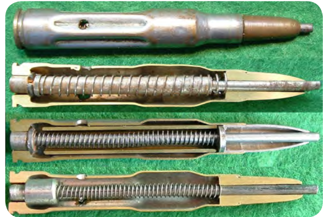
Fig. 15 - Hollifield Dotter cartridges for Model 1903 and 1917 rifles showing variations in construction details (Courtesy International Ammunition Association)
