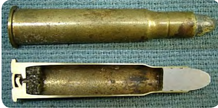
Fig. 26 - Sectioned Frankford Arsenal conical bullet gallery practice cartridge.
