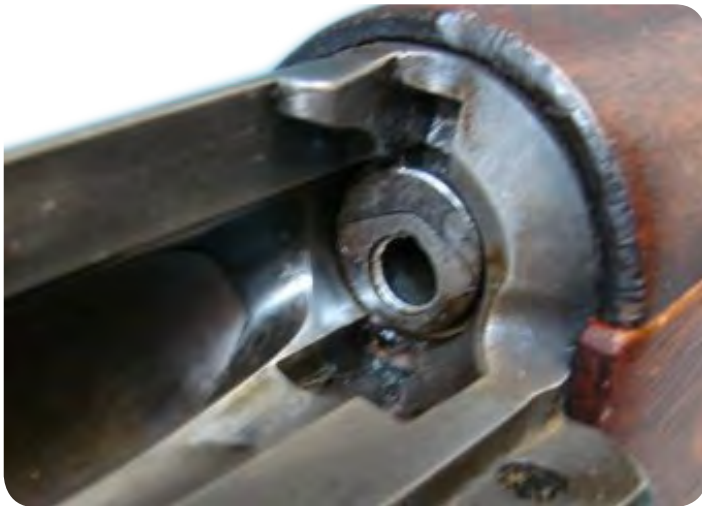
Fig. 33 - Springfield Armory Model 1898 Gallery Practice rifle in .22 caliber showing the extractor plate arrangement.
