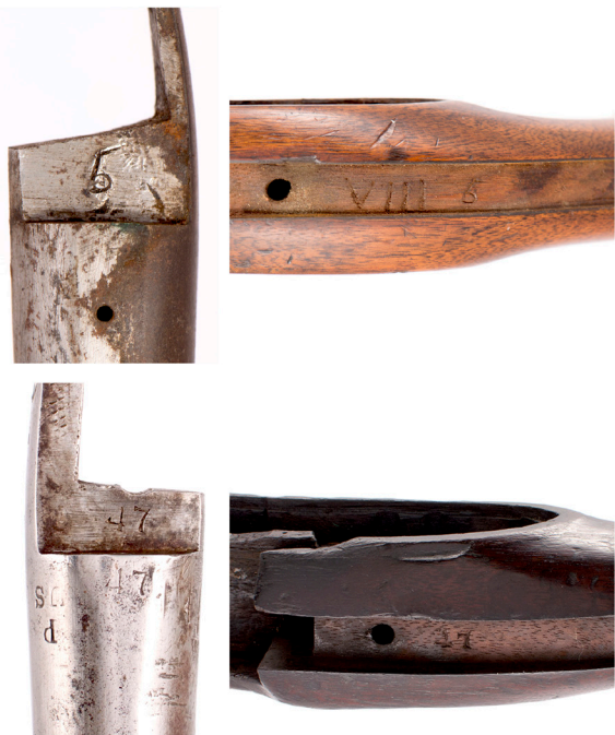
Figure 29. Example of numbering used to mate the barrel, breech plug and stock in pin fastened pistols. Number 5 stamped with a "c" and "I" to make the number observed on a privateer example (top) and iron banded example stamped with number 47 (bottom).
