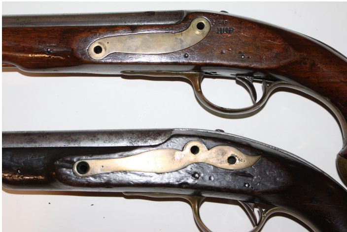
Figure 13. Comparison of side plates on North Pattern 1808 and 1811 pistols.
