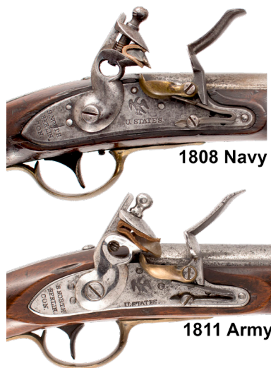
Figure 12. Comparison of lock plate found in North Pattern 1808 and 1811 pistols.
