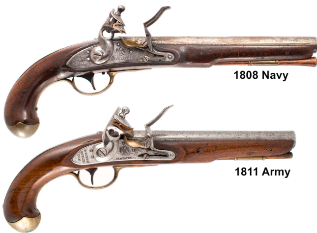
Figure 14. Comparison of trigger position inside the trigger guard on North Pattern 1808 and 1811 pistols.
