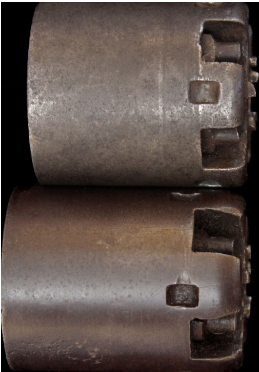
Figure 24. Both revolvers are .36 caliber, but the difference in powder charge was substantial.
