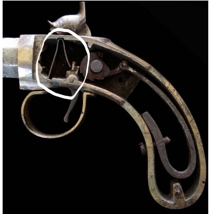
Figure 14. Note the “U” shaped springs used for the trigger return and even for the mainspring.
