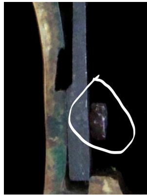
Figure 27. The inaccessible screw head found in Number 2.
