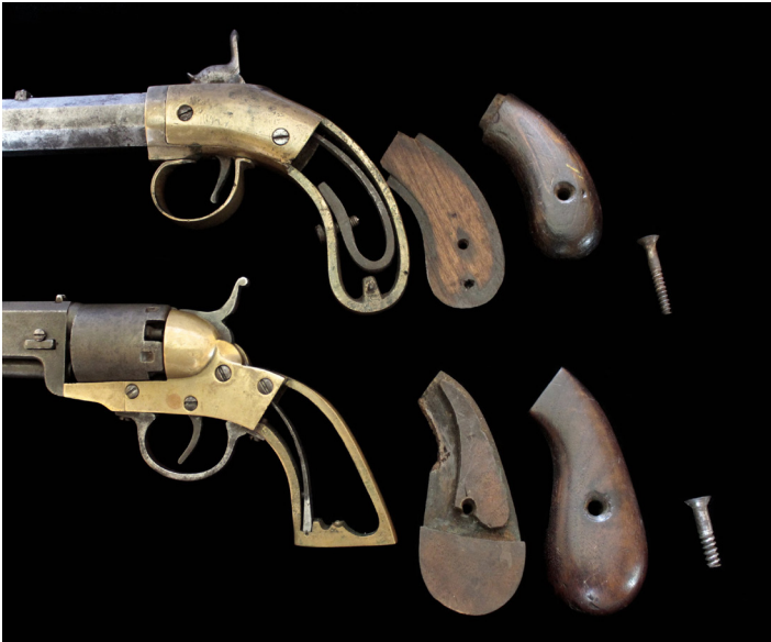
Figure 12. Both the Garrett Type II Pistol and their revolver had hand tooled, rounded slab grips fastened together by passing a wood screw through one countersunk slab grip and screwed into the opposite slab.
