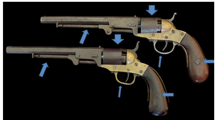
Figure 15. Note the slight differences between revolvers 1 and 2, including the rammer lever, the cylinder, the trigger guard and the reversed grip screw.
