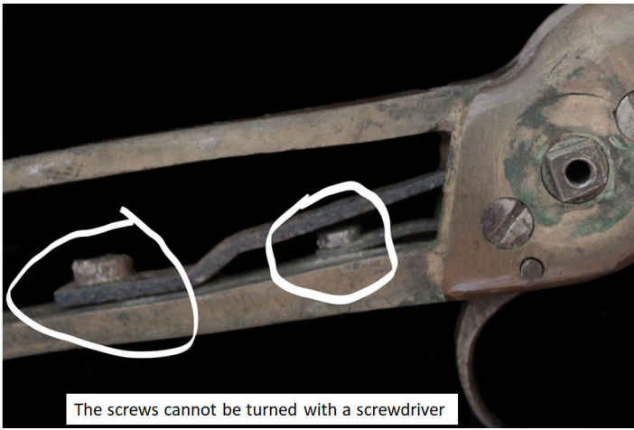
Figure 26. Both the Tarpley Carbine and Revolver Number 2 have the oddity of having mainspring screws with slotted heads, though neither can be accessed by a screwdriver.
