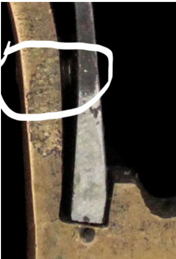
Figure 20. A new problem was created, now the screw that was moved from the top of the side plate is blocking the mainspring from compressing, thus preventing the hammer from going to full cock. The answer, file the screw's diameter in half!
