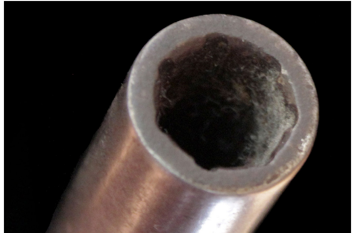
Figure 6. Note the seven broad lands and seven narrow grooves. This style of rifling is a Guilford County Gun maker Hallmark.
