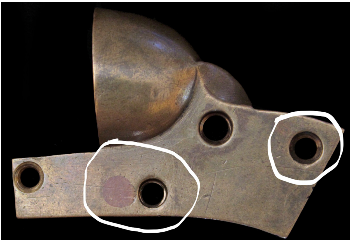
Figure 16. The side plate of Number 1 would not work where the center hole was originally drilled. Rather than cast a new plate, the Garrett's chose to fill the hole and re-drill.
