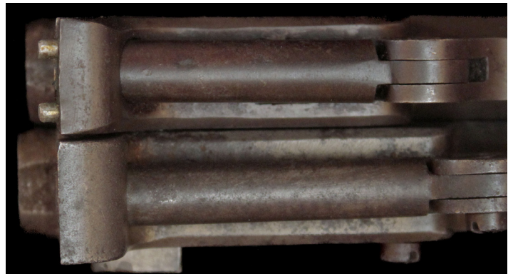
Figure 23. Number 1 above set the steady pins in the frame, in Number 2 the pins were set in the leg.
