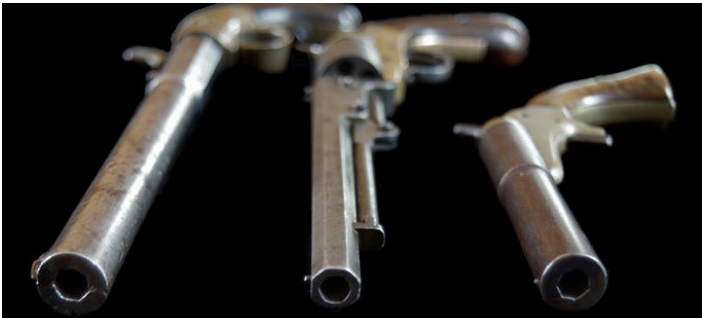
Figure 13. J. and F. Garrett gave the Tarpley, (not shown) and the Type I, Type II and Revolvers 1 and 2 the seven broad lands and seven narrow grooves of rifling commonly found in Guilford County Rifles.
