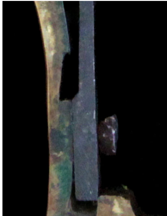
Figure 21. Creating a dovetail for an adjustment wedge also created a weak place.
