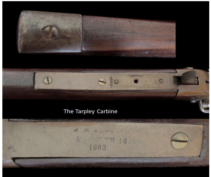
Figure 29. Tangs on the Tarpley Carbine.
