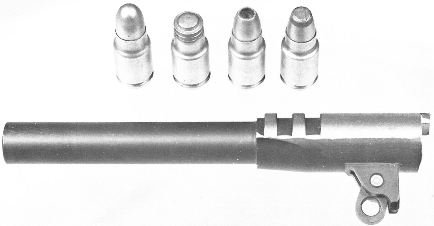
Figure 41. Whitney .38/.45 sub-caliber barrel
