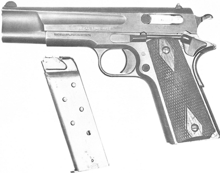
Figure 2. Later Springfield Armory .22/.45 conversion unit.
