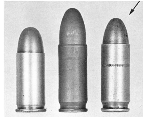
Figure 3B. In this illustration the cal. .30 Pedersen cartridge is on the far right and the .32 ACP pistol cartridge on the far left. The center round is the French 7.65 mm. Long developed after World War I. By coincidence it is practically identical with the .30 Pedersen round.
