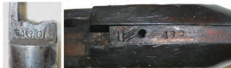
Breech plug marked on left side and backstrap channel of stock marked with "430". The additional "II" on the stock is often associated with markings for percussion conversion.
