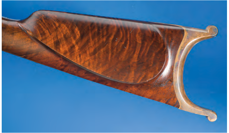
Custom check piece on left stock. Rifle style crescent butt plate, noted in the Sharps order book as "broad rifle butt"
