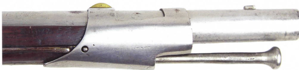
Figure 5. Forward barrel band of 1798 U.S. contract musket with button ramrod (Gilbert).
