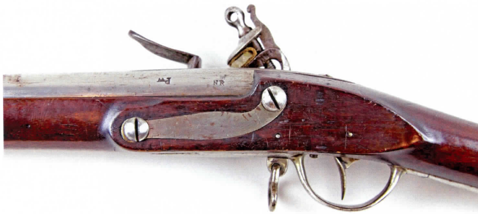
Figure 3. Barrel proofs for a 1798 contract musket, note the “Pw,” which stands for proofed by Decius Wadsworth.
