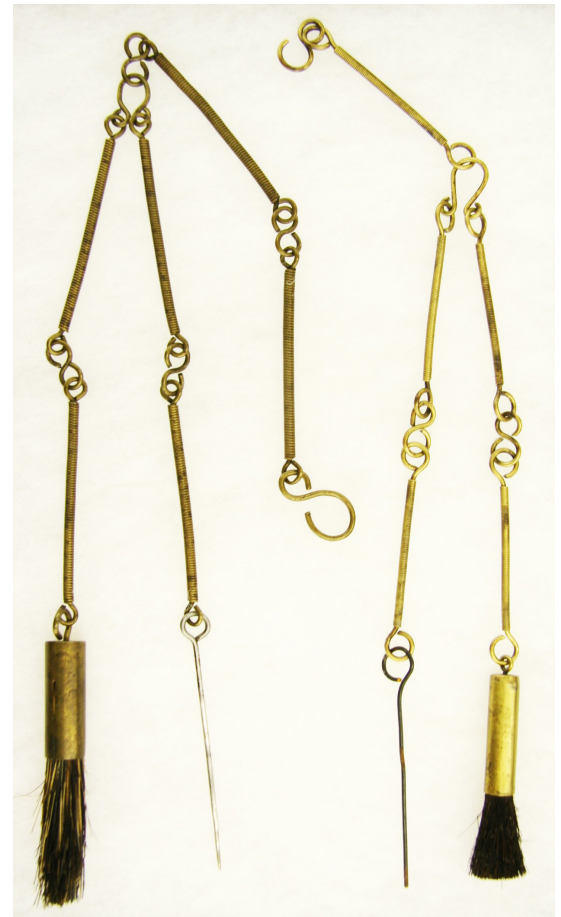
Fig. 6 - Although similar, the links are shorter (2 5/8 in.) on the example at right than the one at left (2 7/8 in.) It also has only one link above where the set are joined by a curled wire connector. The one at right may represent the pattern adopted in 1827. Courtesy the late Phil Leveque and Fred Gaede.
