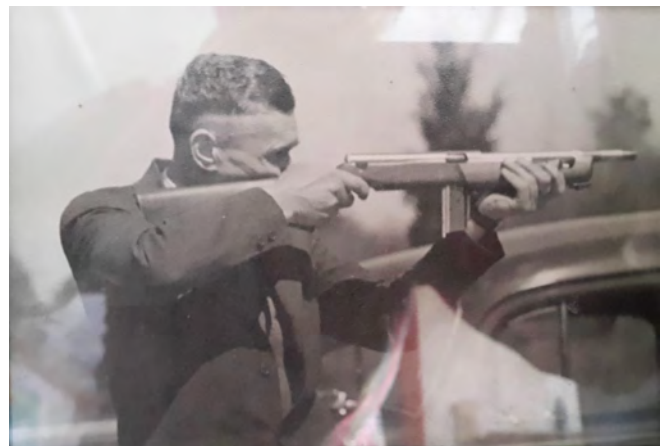
Figure 15. A family photo of Eugene Reising, circa 1938-39, with a prototype of his Model 50 Submachine Gun. Notice the actuator bar is on the right forward side of the stock. Image Credit: Clifford Cousens
