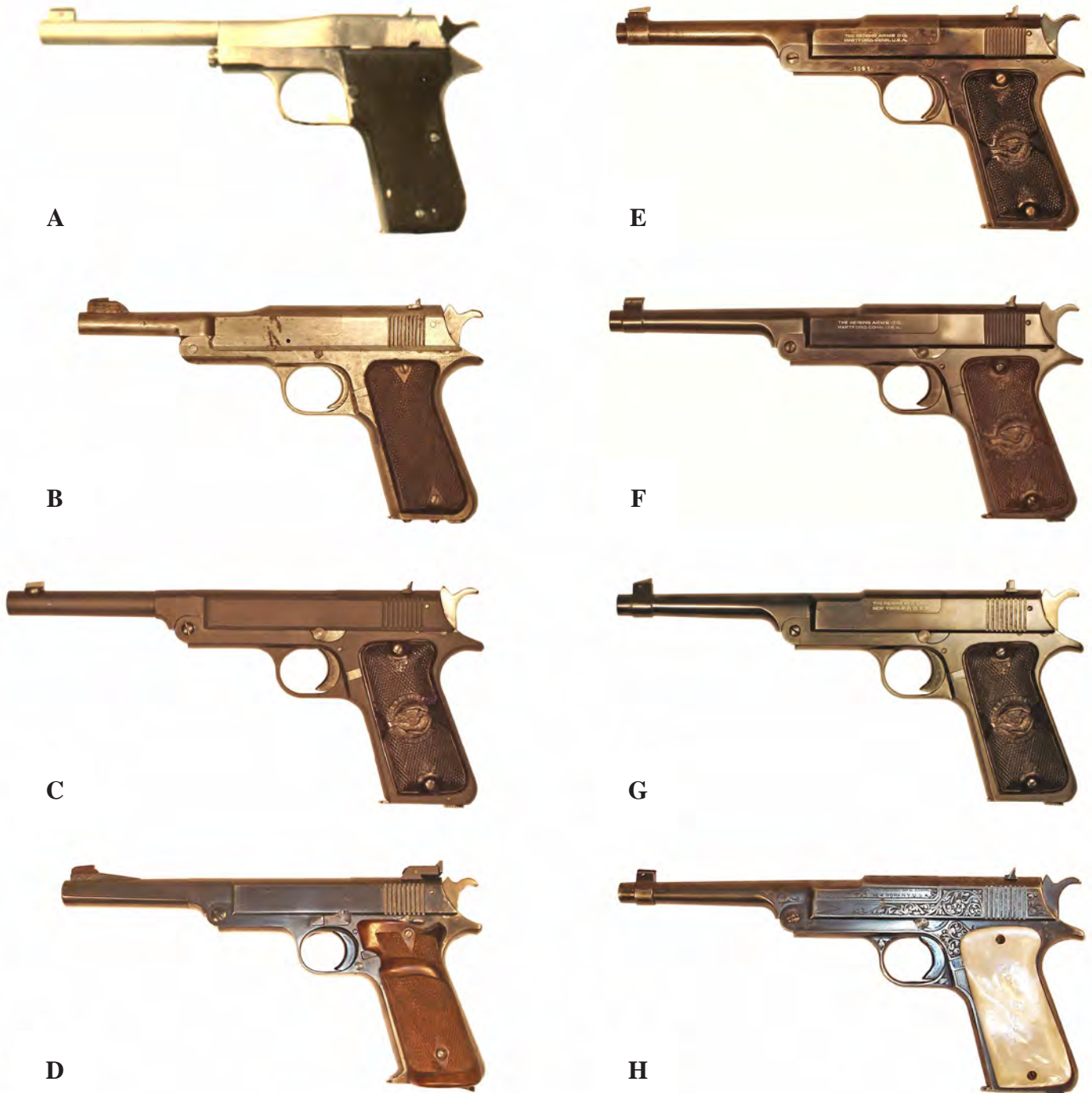
Figure 5. Prototype Reising .22 Pistols A) Original 1st prototype, patent filed in 1915, approved 5/16/16. Patent was for magazine disconnect, first firearm to incorporate this feature. Was to be marketed under Dalton Arms Corp., but none produced B) 2nd prototype, patent filed in 1919, approved 10/25/21. Taking form of production pistol. An early pistol was tested by Springfield Armory in 1920. C) EXP-1 November 1928 prototype. Patent filed in 1928, approved 1/3/32. Post commercial manufacturing prototype. D) EXP-3 Another post commercial manufacturing prototype. Heavy barrel target model, adjustable rear sight, slide stays open after last round. E) Reising Arms Company pistol, early Hartford, Conn. production gun. Wide front sight blade, push button barrel lock, ability to load single shots, tip up barrel, 12 round magazine. F) Later Hartford, Conn. production gun. Finer sight blade, toggle type barrel lock, serial number relocated to front grip strap. G) Reising Manufacturing Corp, New York marked pistol. Finer sight blade toggle type barrel lock, serial number relocated to front grip strap. H) Reising Manufacturing Corp. Deluxe Model. Pearl or Ivory grips, frame, slide, and barrel engraved, came in deluxe case with Reising cleaning rod.
