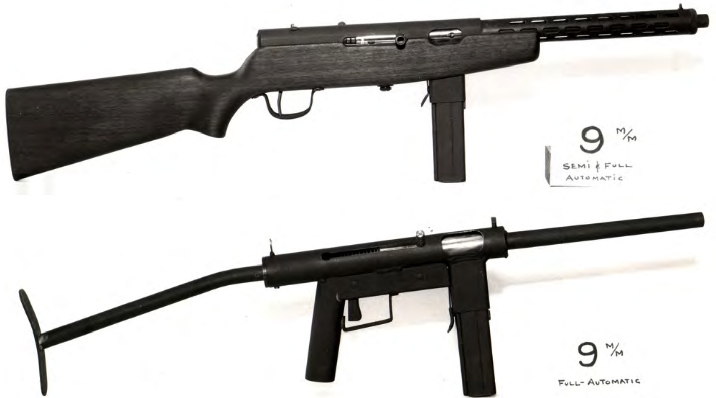
Figure 31. Two Eugene Reising designed 9 mm submachine guns of the late 1950's to early 1960's that never saw production by H&R. The first was nicknamed "Special Forces" (Top) and the second was nicknamed "Assault" (Bottom)
