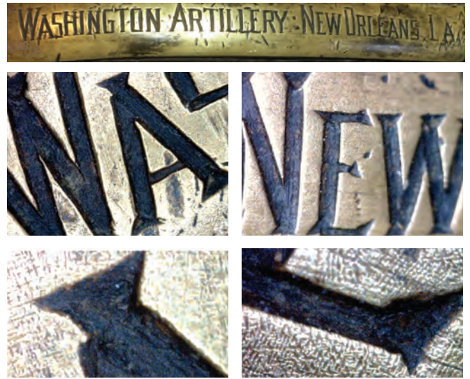
Figure 2. Washington Artillery – Note the dent under the “A” in Washington has been cut through.
