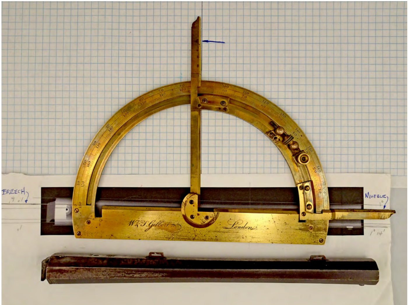
Figure 9. Vernier protractor measuring angle between bore tangents at breech and muzzle of a bent Wogdon barrel from a full-scale neutron radiograph.
