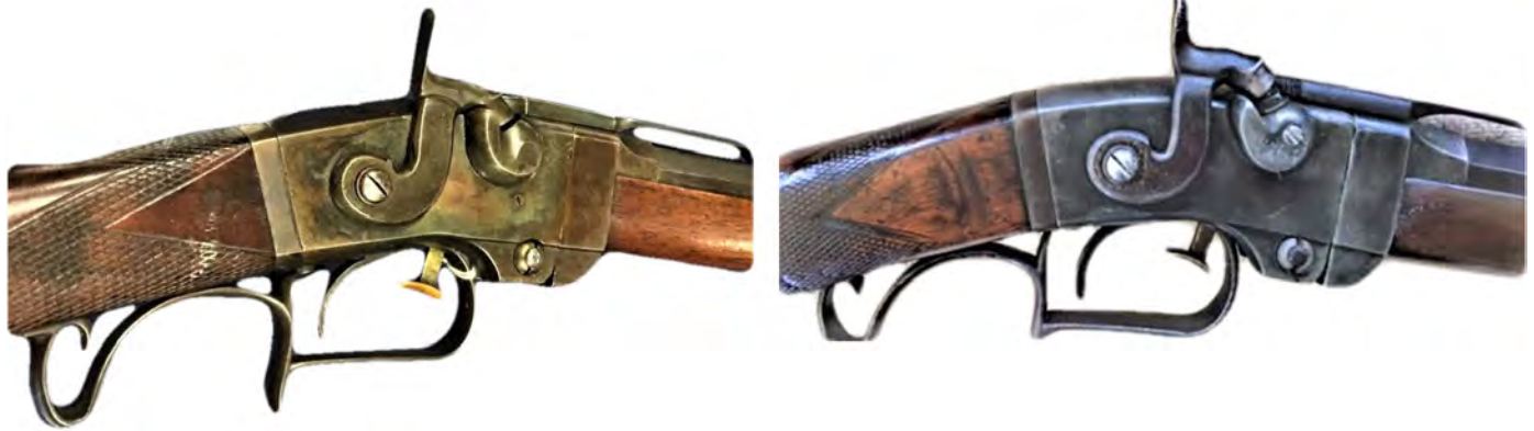
Figure 19. Details of the receivers of Model 1860 Smith patent carbines showing details of the sloping receiver, the characteristic trigger guard and examples of stock checkering. The carbine on the left shows a nipple bolster without clean-out screw (Private collection) and the carbine on the right shows the nipple bolster with one (Don Dietrich collection).
