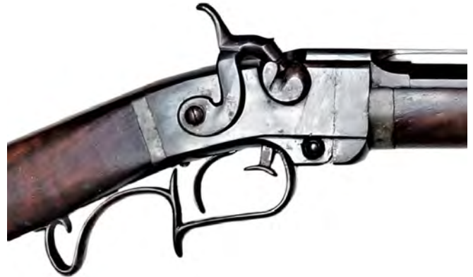
Figure 17. Detail of receiver of Model 1860 production Smith patent carbine. (Hubert Lum collection).
