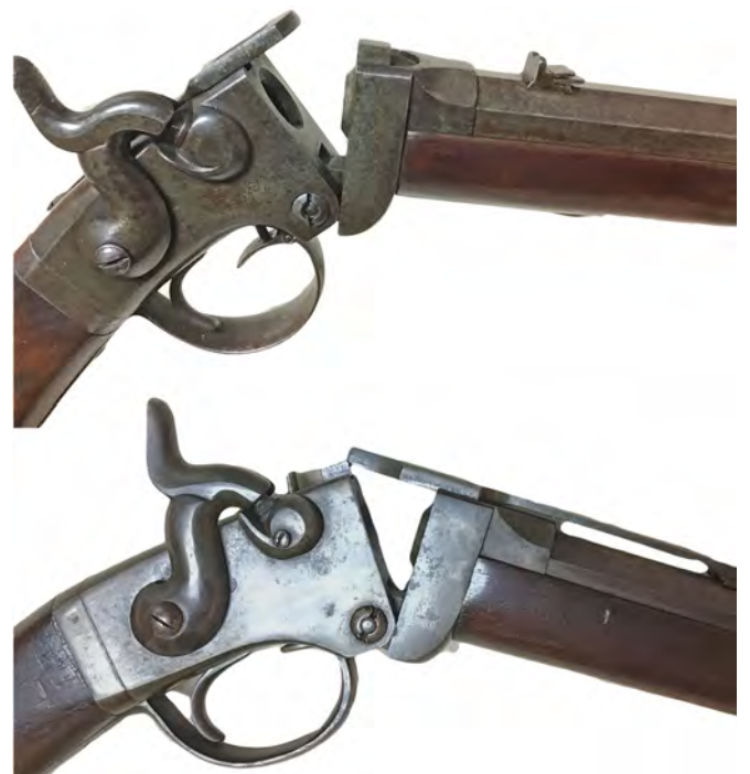
Figure 11. Details of Model 1859 carbines showing the different arrangements of the locking strap as described by the Army Board at the Washington Trials in 1860. Top carbine has the locking strap over the receiver (Hubert Lum collection). The bottom carbine has the locking strap over the barrel (Author's collection)
