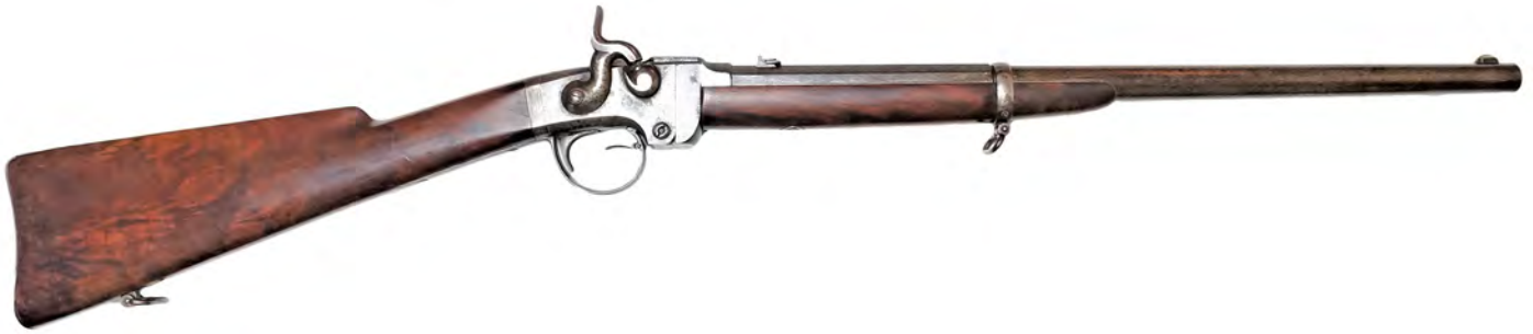
Figure 8. Model 1859 military style carbine with spring closing strap over the receiver (Hubert Lum collection).
