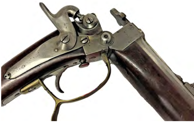
Figure 6. Smith prototype carbine showing the breech opened (Collections War Heritage Institute, Inv 11746).
