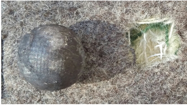
Figure 4. Ball with a plain woven cloth imprint retrieved from the ballistics gelatin.
