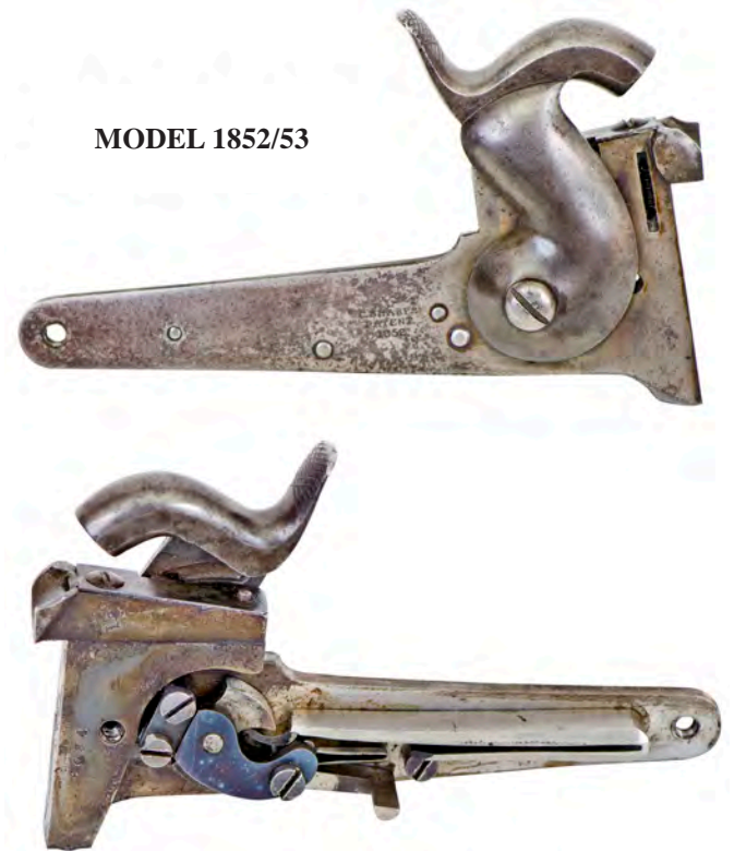
Figure 8. Model 1852/1853 Lock. This lock incorporates Sharps' pellet primer. Small primer disks were loaded into the lock via a copper tube, which held twenty-five to thirty-two primers. The primary concern expressed was that a percussion cap could not be used once the disks were loaded, a defect corrected with the introduction of the Lawrence pellet primer which incorporated a "cut-off" in the Model 1859. A second comment was that the disks were difficult to load in cold weather with numb fingers.
