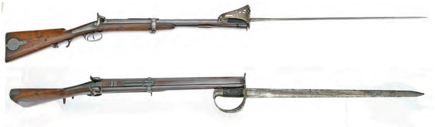
Figure 8. The Jacob rifle with its mounted bayonet, having a 30 inch blade and a “Scottish cut-out like hilt”, has an incongruous, unbalanced appearance.
