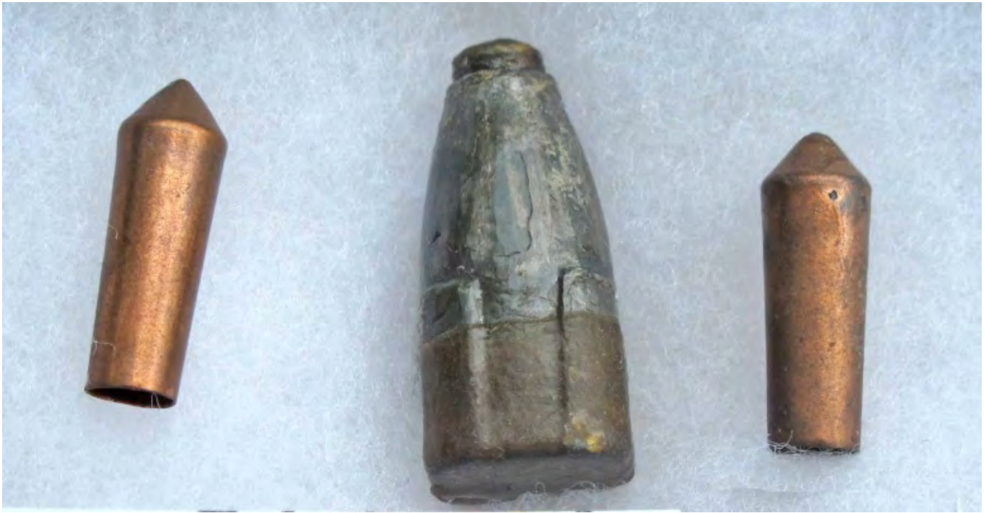
Figure 13. Jacob explosive bullet with copper tubes of fulminate of mercury. To detonate on contact to explode caissons, as opposed to the timed fuse of a Gardiner bullet.
