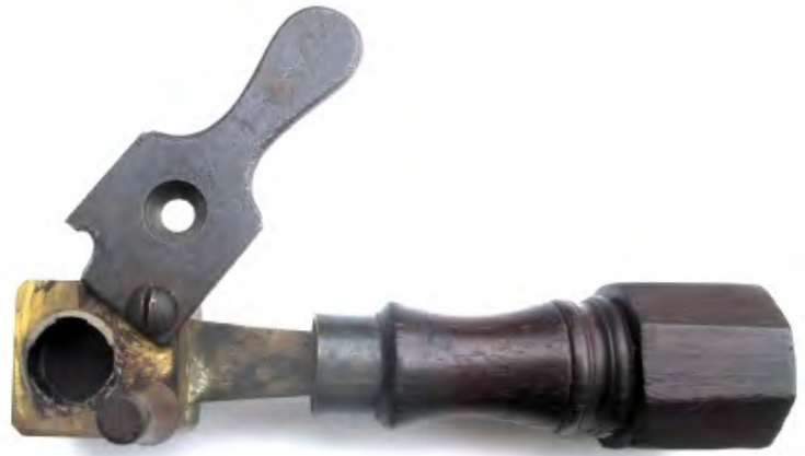
Figure 9. Daw-style Jacob bullet mold casting a .563 inch caliber bullet (.604 inches to the lugs).
