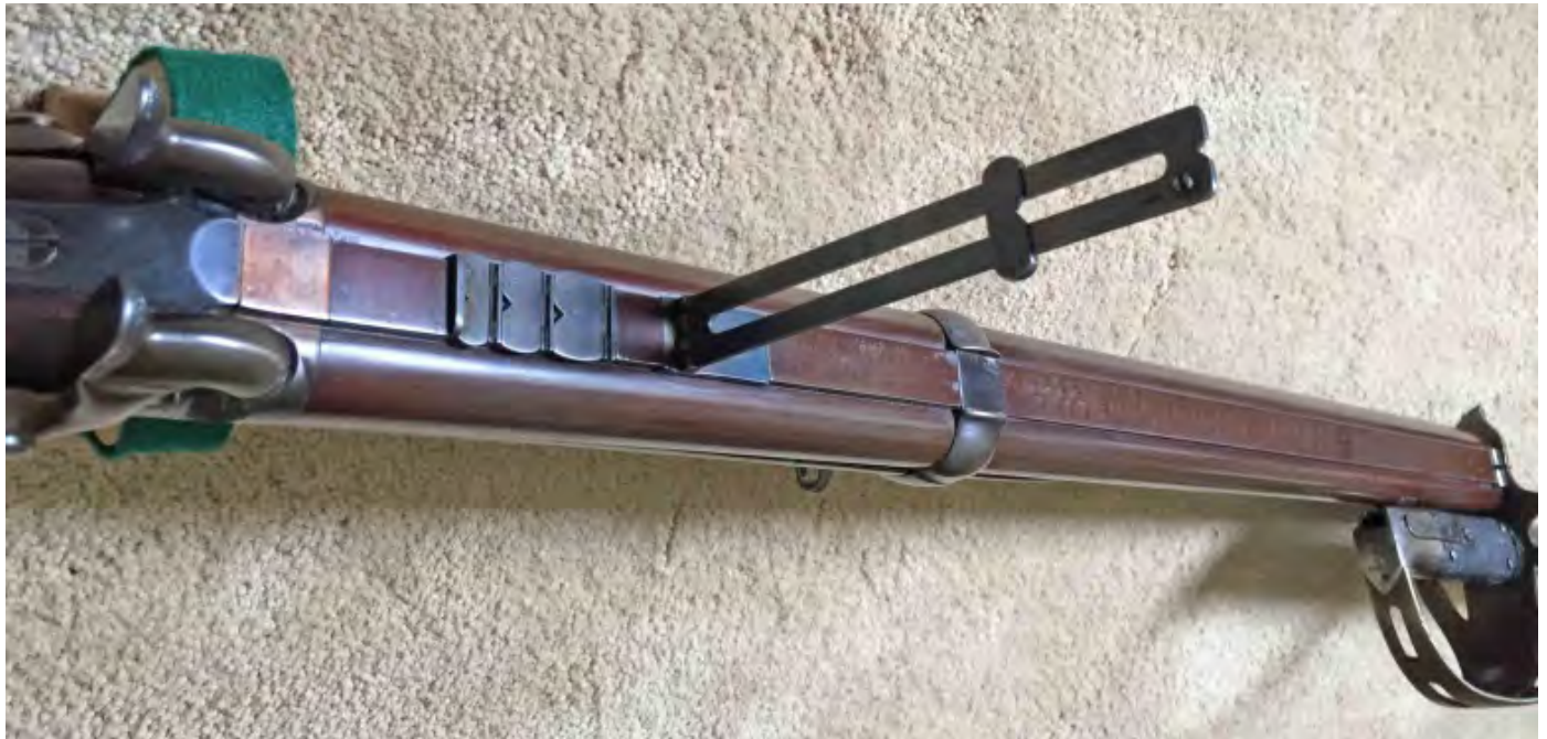
Figure 4. The Jacob rifle's rear sight has 3 leafs graduated from 100-200-300 yards, plus a 5 inch ladder sight to 2,000 yards!
