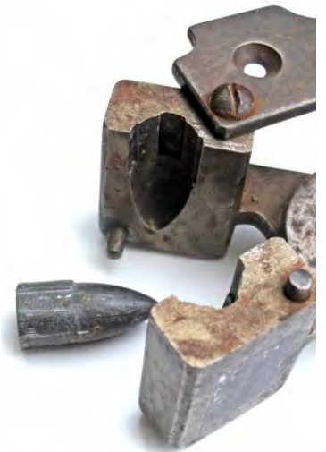
Figure 9. Daw-style Jacob bullet mold casting a .563 inch caliber bullet (.604 inches to the lugs).
