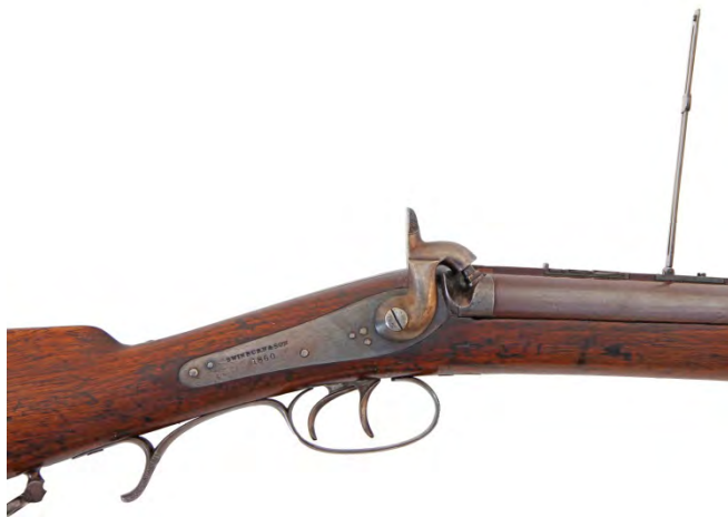
Figure 6. The back-action locks have robust military hammers and are marked “SWINBURN & SON/1860”.
