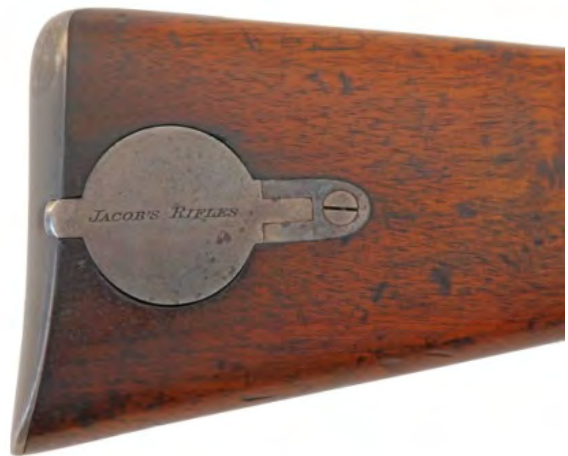
Figure 7. The spring-loaded patch box in the right buttstock is marked “JACOB’S RIFLES”.
