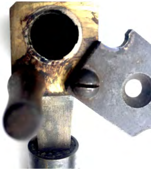
Figure 9. Daw-style Jacob bullet mold casting a .563 inch caliber bullet (.604 inches to the lugs).
