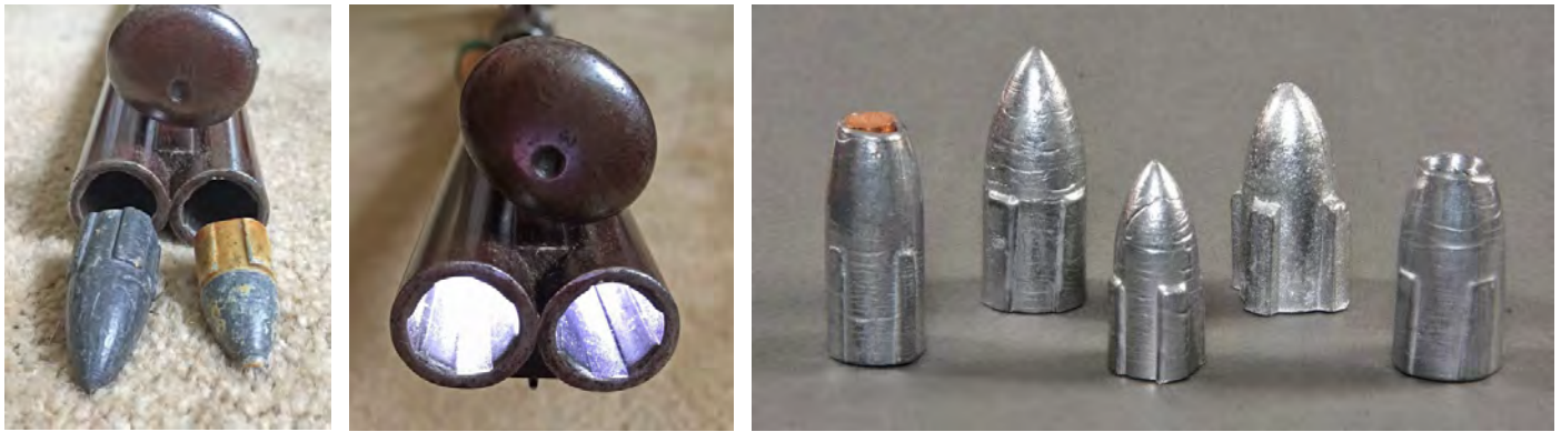
Figure 3. The deep 4-groove rifling (3/4 turn in 24 inches), with its lands of equal width to the grooves, with bullets cast with 4 lugs to engage the rifling.
