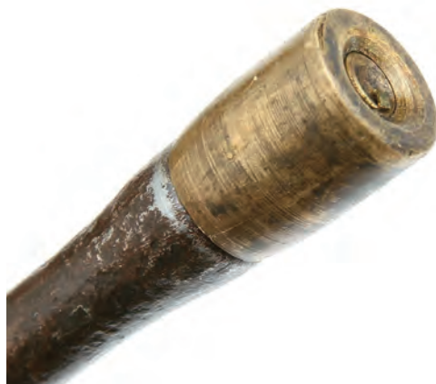
Figure 5. Concave tip of the ram rod for seating bullets with an explosive copper tip.
