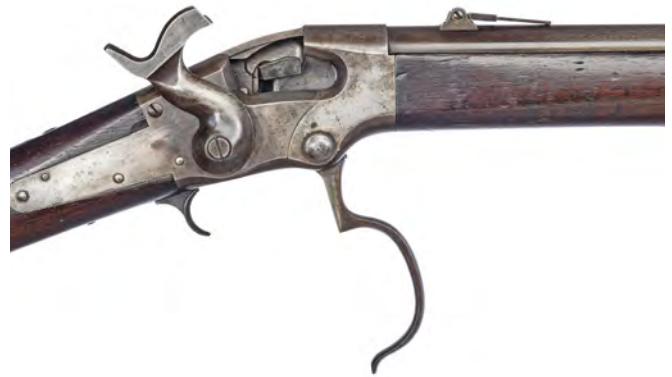
Figure 3. Compare this photograph of the Ball Patent design with the drawings of Figure 2. The Ball breechloading mechanism suffered from the same limitation as the Spencer carbine design: it was limited to the use of short cartridges of limited power. (Courtesy the Institute for Military Technology, Michael Fullana photo).
