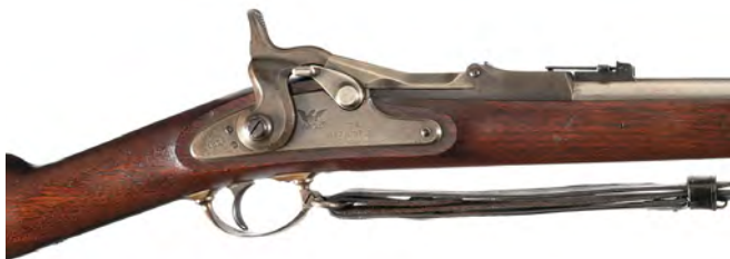
Figure 13. The standard Springfield Model 1868 Rifle has a longer receiver than on all subsequent Models 1870/73/84/88. (George Moller Collection, courtesy Rock Island Auction Co.).
