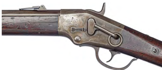
Figure 5. The Ball rifle of Figures 3 & 4 is marked in six lines, "E. G. LAMSON & CO. / WINDSOR. VT U.S. / BALLS PATENT. / JUNE 23.1863 / MAR. 1 ____." The rotating magazine cutoff lever obscures the rest of date "15, 1864," the reissue date of the first patent. (Courtesy the Institute for Military Technology, Michael Fullana photo).
