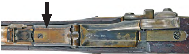
Figure 14. This is the model rifle with the “Lamson extractor” made at Springfield in mid 1868. Note how the flat spring spans the entire receiver and the ejector disc is located on the right side of the breechblock pivot pin. The breechblock is marked with the U.S. eagle and “AUG 1868.” (Courtesy the Springfield Armory National Historic Site, SPAR 5658).
