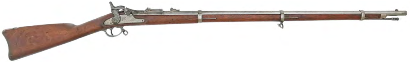
Figure 7. This example of the Lamson-Ball trapdoor musket retains the overall length of the original Springfield Model 1864 Rifle Musket, but the barrel length in-the-bore is now 37 inches. Its barrel is relined to .50 caliber like the Springfield Model 1866; it's chambered in caliber .50-70 Government. This is one of two known examples, the other being a caliber .58 rimfire version that had the breechblock pivot pin affixed to a strap on top of the barrel. (Author's collection and photo).
