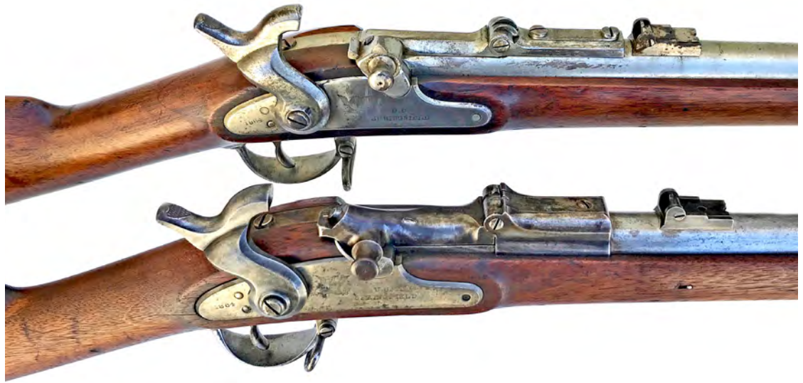
Figure 10. The overall breech design of the Lamson-Ball musket (bottom) is copied from the prototype “sliding breech” trapdoor design of Hiram Berdan (top). Berdan was working at Lamson’s factory in 1866, to develop his trapdoor designs, only later to move to the Colt Fire Arms factory. (Author’s collection and photo).
