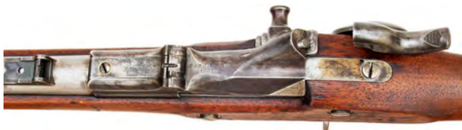
Figure 12. The breechblock of this .50 caliber version of the Lamson musket is marked in two lines merely "PAT JAN 1 / 1867." The flat spring of the Lamson-Ball ejector is inset into the top of a cylindrical band which encircles the barrel at the chamber. (Author's collection and photo).
