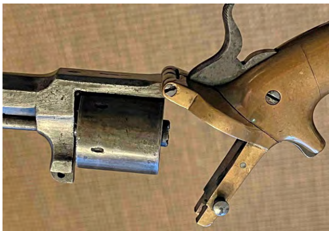
Figure 6. A brass-framed Lucius Pond Belt Revolver, serial number 4508. the robust and well-designed barrel hinge. (Author’s collection)
