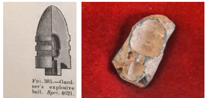
Figure 1 Left: Lithographic illustration of Gardiner explosive bullet; Right: Sectioned Gardiner explosive bullet found at Gettysburg - showing fuse hole and explosive powder charge chamber.
