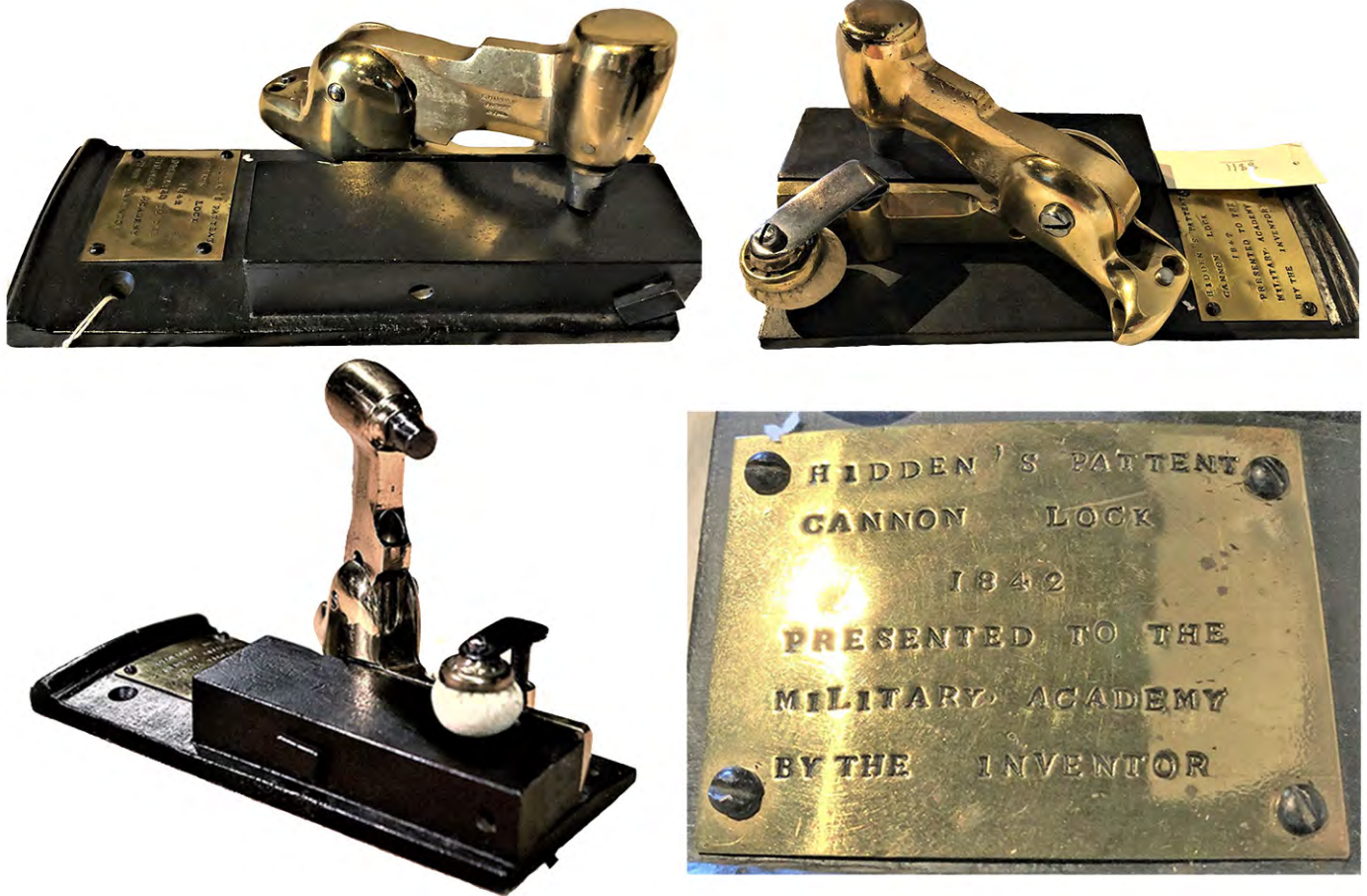
Figure 2. Overall image of Lock No. 11011, hammer closed, E. HIDDEN / PATENT / PENDING mark on neck of the hammer (upper left). Hammer closed, other side of lock (upper right). The hammer is open and the closure cushion for the vent is obvious (lower left). 1842 presentation plaque for this lock (lower right).
