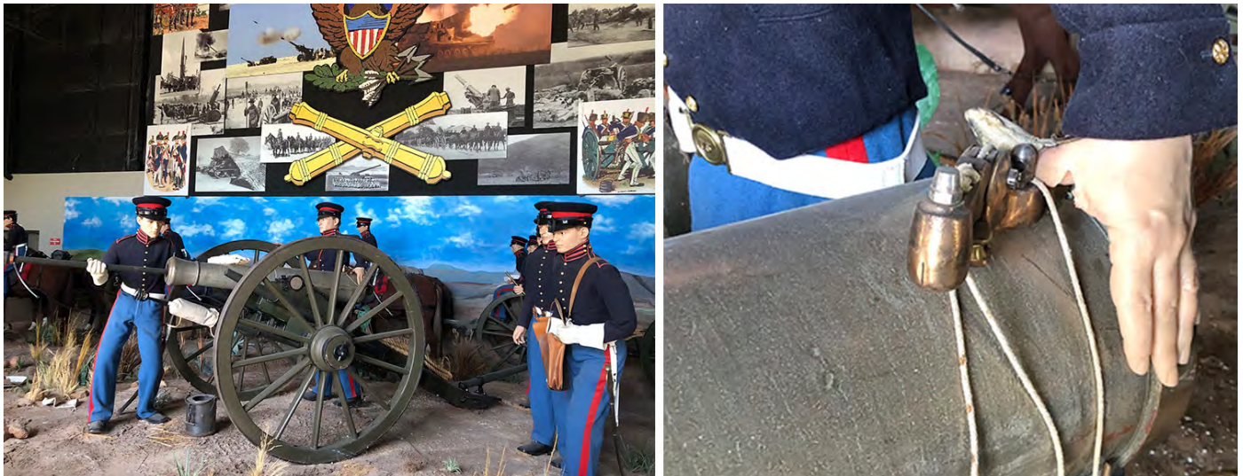
Figure 1. Part of the diorama at the entrance to the U.S. Army Artillery Museum, showing a section of artillery with reproduction Hidden 1842-patent field artillery cannon locks in place (left). Close up of a Hidden lock mounted on a M1841 tube, ready for the lanyard to be pulled and the charge ignited (right). Unless otherwise noted, all illustrations courtesy Gordon Blaker.
