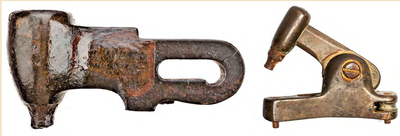
Figure 2. A field-recovered sliding hammer from a M1842 Hidden cannon lock. Courtesy Jack Melton and The Artilleryman magazine (left). Sideview of a M1842 Hidden lock, without a vent closure device (right).
