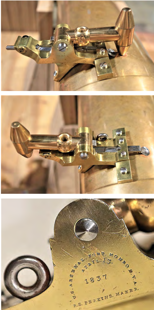
Figure 7. Overall view of a unique cannon lock designed by R.S. Perkins. Note the double-headed hammer, and the vent cover retracted. The likely machinist’s name “J. COUCH” can be seen at the bottom edge of the lock (top left). Perkins’ lock opened, with the vent cover automatically extended over the vent (top right). The marking of Perkins on the lock body, with an indication the lock was at Ft. Monroe, Virginia in April of 1837 (bottom).
