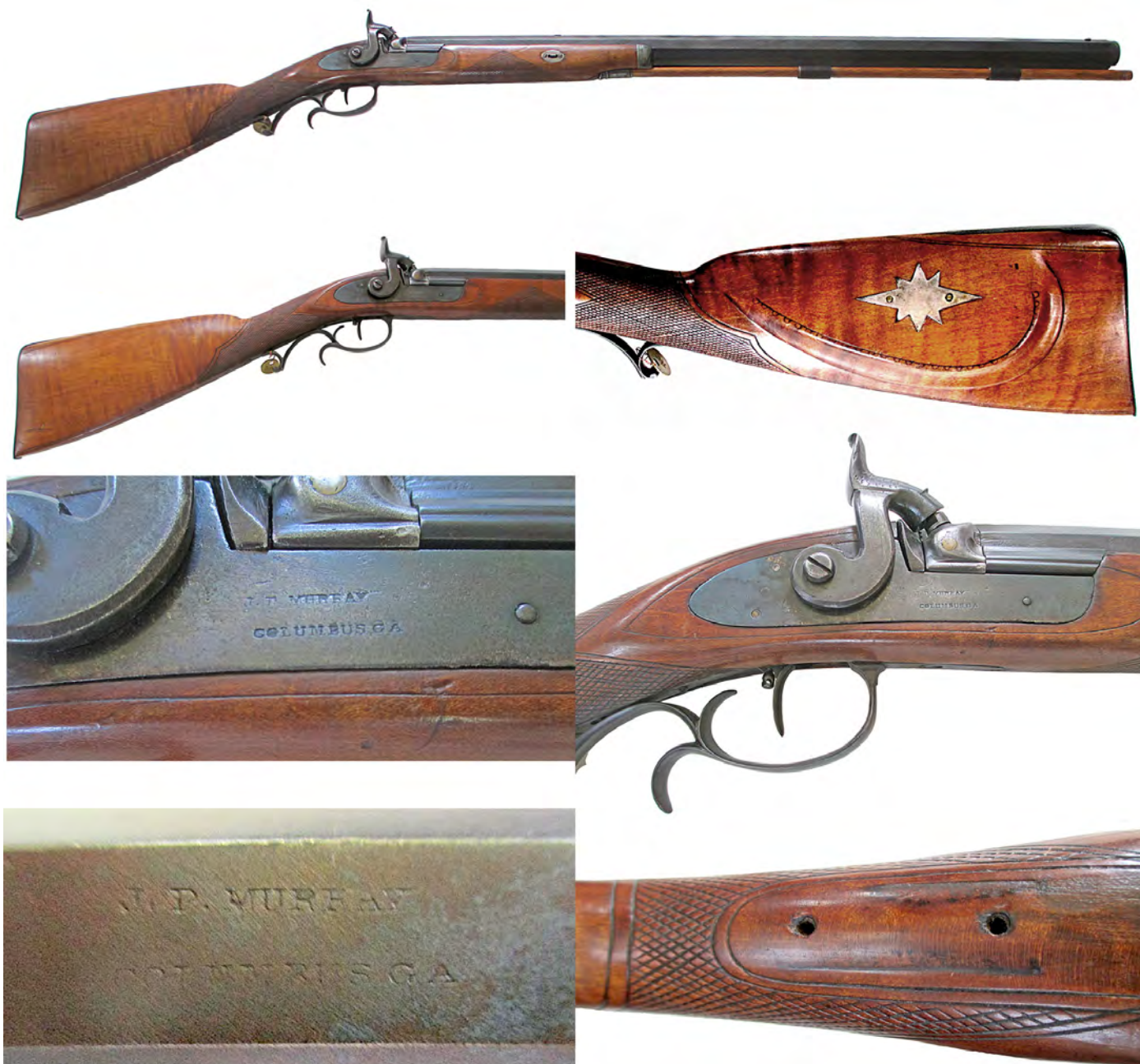
Figure 2. Half stocked pre- Civil War .50 caliber percussion rifle made by J.P. Murray of Columbus, Ga.
