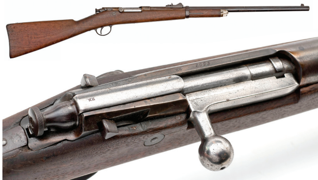
Figure 14. Second model bolt action Winchester Hotchkiss carbine. Note the magazine cutoff (right tab) and safety (left tab) has been moved to either side of the bolt at the rear of the receiver. Photos courtesy of Jack Lewis.
