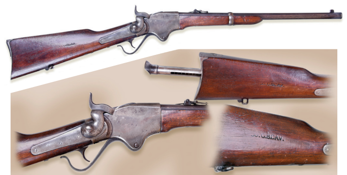
Figure 2. Spencer carbine. Note the tubular magazine that is fed into a receptacle in the butt plate. Photo courtesy of Ron Paxton.
