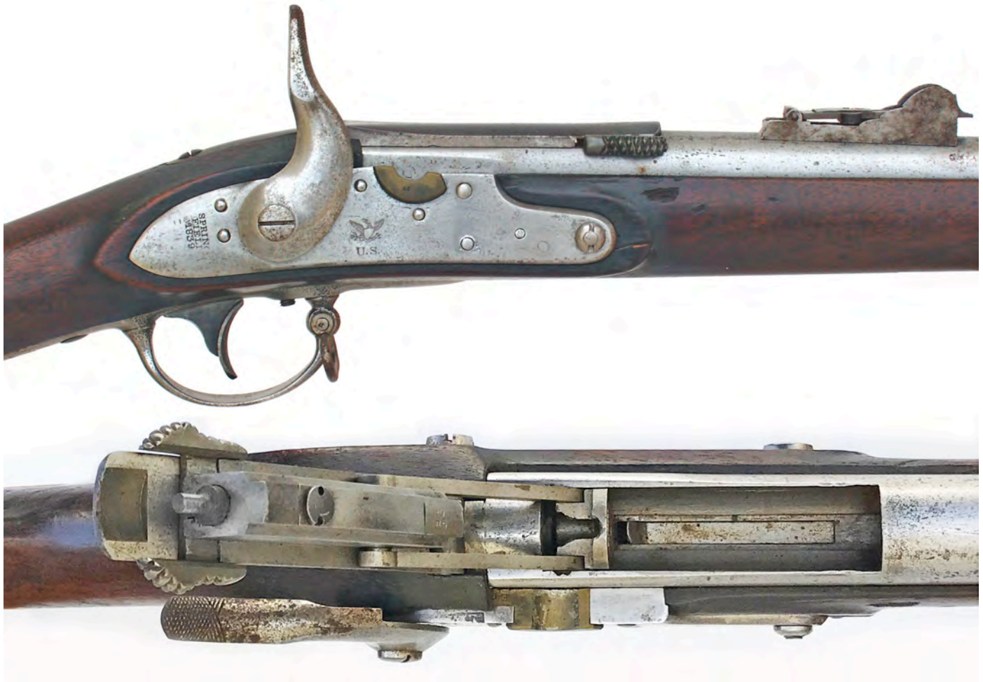
Figure 11. Close-up photographs of the open breech of the .69 caliber musket of Figure 2. The top photo shows the lockplate forward through-bolt which is held by an external nut — typical of all production muskets. The lower photograph shows the extractor lever at the base of the slot. (Author's collection and photo)
