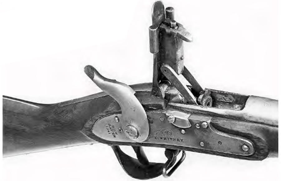
Figure 9. The .69 caliber musketoon made by C.H. Munck shows the sliding breech design which Morse finally developed, combining both of his patents. It is an E. Whitney Model 1822 musket dated 1841; its total length is 41½ inches and the barrel is 231/16 inches long in-the-bore. (SPAR 4709, Springfield Army National Historic Site, Photo by H.M. Madaus)
