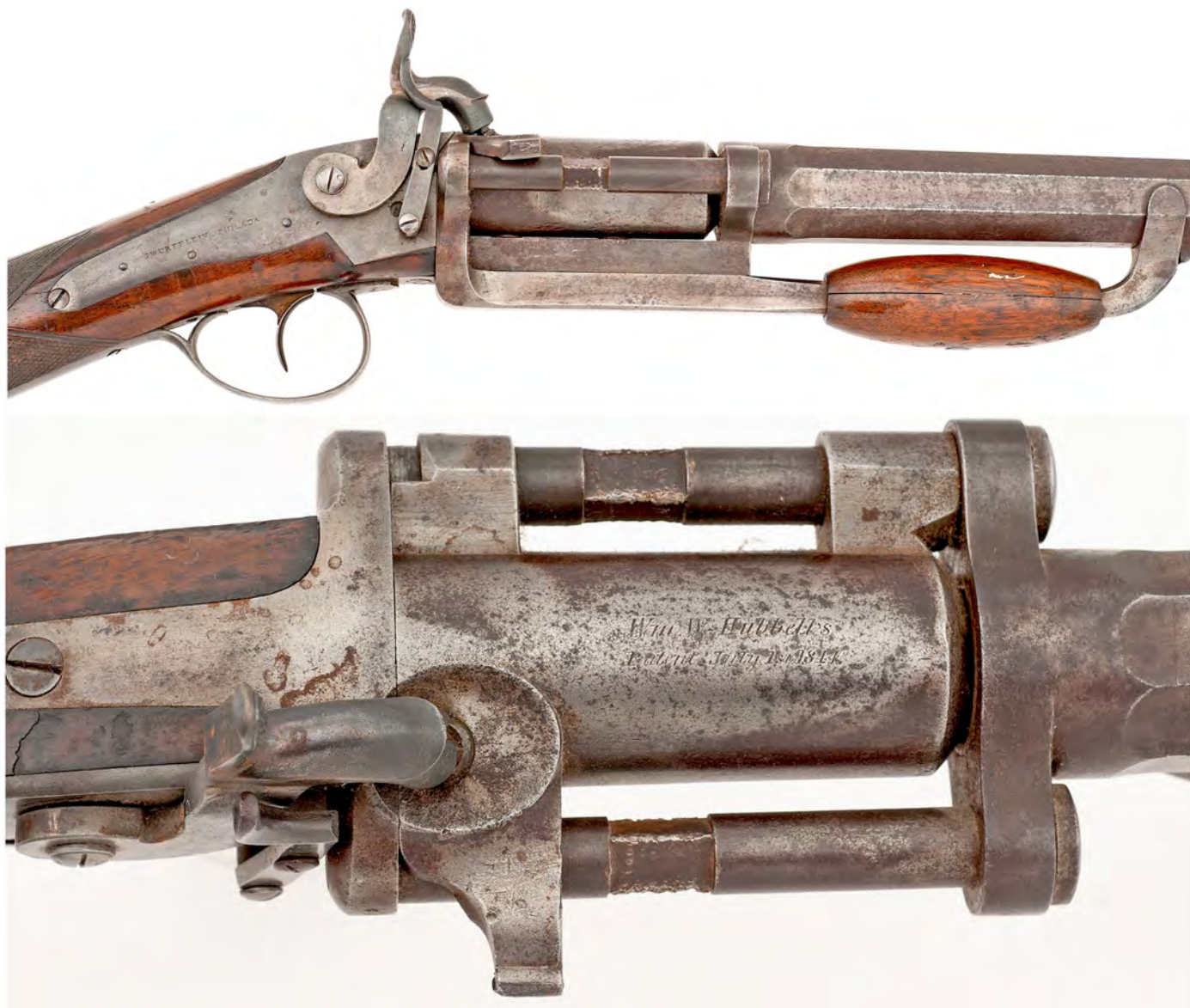
Figure 20. This is an example of Hubbell's first design for a breechloader, with its leftward rotating chamber. It is engraved on the top of the chamber "Wm.W.Hubbell's / Patent July 1.1844 " in two lines. (courtesy Cowan's Auctions)
