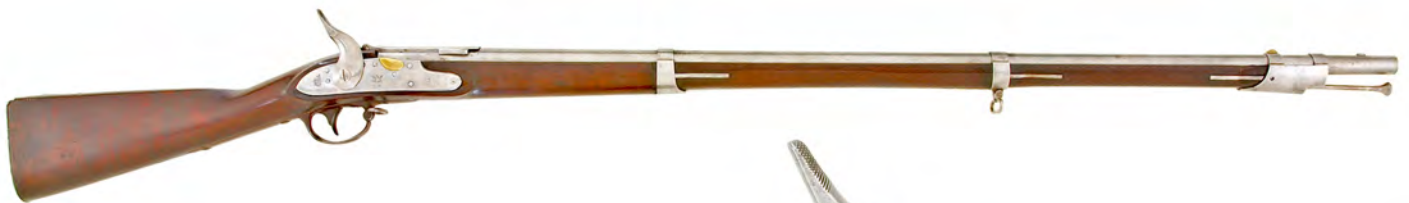
Figure 10. This Morse alteration musket is stamped “1” on the major breech parts. It is likely one of the first two sliding breech models made, and the one returned to the Springfield Armory in May, 1859, for use as the official model. It is smoothbore and lacks a rear sight. Note the smooth contour of the finger latch “ears” on the breech latch/firing pin; production muskets had this part knurled. (Courtesy Heritage Auctions)
