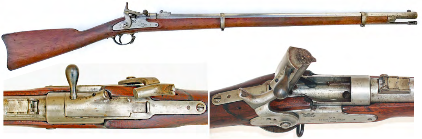
Figure 25. This is a Van Choate prototype rifle of his "reverse-trapdoor" type, the design of which is illustrated in Figure 24. The .58 caliber barrel is 30½ inches long in the bore. The rifle is assembled from a shortened Springfield Model 1863 rifle musket. On this prototype rifle the firing pin angles downward from the hammer to the center of the face of the breechblock. When the breechblock is opened upward a link draws the extractor rearward; there is no ejector and the rifle must be inverted for the case to fall out. Note the unique contour of the undated lockplate. The short breech opening limits the length of the cartridge; the chamber accepts the short .58 Gatling centerfire cartridge. The breech system is finished in-the-white. The breechblock is stamped lightly "S.F. VAN CHOATE / INVENTOR" in two lines. (Institute of Military Technology collection, photos by author)
