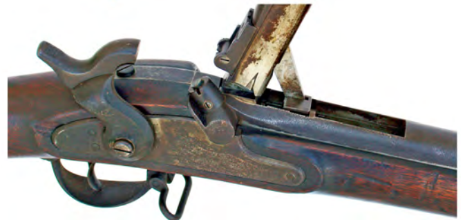
Figure 22. This Hubbell 1867 musket conversion is the only known example of his design; the iron barrel and furniture was originally finished bright but now have an overall deep patina. The barrel/breech system retains the musket's original 40 inch length; the in-the-bore barrel length is 35½ inches. The barrel is chambered for the .50 Government (.50-70) cartridge. It is a conversion of a "SPRINGFIELD" marked Model 1864 Rifle Musket that has the standard inspectors' cartouches on the stock, which indicates the use of a surplus military arm. The top of the breech lever is marked across the front end "W.W.HUBBELL / PATENT / JUNE 18,1867 / PHILADA PA" in four lines. (Author's collection and photos)
