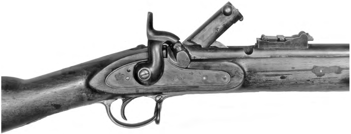
Figure 27. This example of Van Choate's second-type conversion is made on a standard British Pattern 1853 rifle musket. The lockplate is stamped "1857 / TOWER" in two lines; the crown over "VR" and the small crown-over-broad-arrow marks denote original British army ownership. The lock parts are casehardened in color, the barrel and rear sight are blued. (Courtesy Chickamauga & Chattanooga National Park museum)
