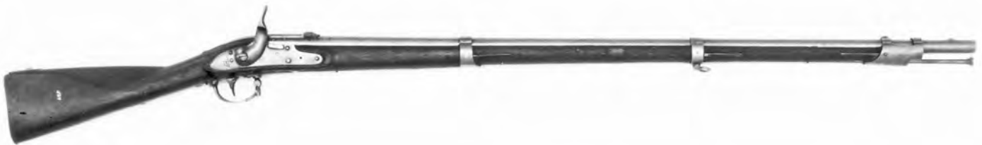
Figure 7. Another of the two Model 1816/22 muskets made on the breech-pin and lid design of patent 20,503. Its smoothbore .69 caliber barrel/breech system is 42 inches long. It is the first Model 1816/22 musket altered by the Washington Arsenal in 1859. The under-stock extractor lever is missing. The forestock shows evidence of charring from the fire at the Springfield Armory in October, 1931. (SPAR 4704, Springfield Armory National Historic Site, photo by H.M. Madaus)
