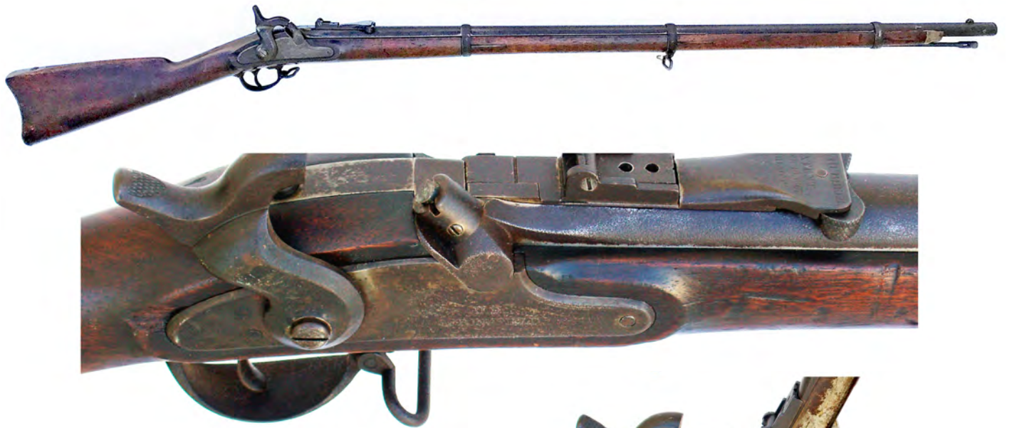
Figure 22. This Hubbell 1867 musket conversion is the only known example of his design; the iron barrel and furniture was originally finished bright but now have an overall deep patina. The barrel/breech system retains the musket's original 40 inch length; the in-the-bore barrel length is 35½ inches. The barrel is chambered for the .50 Government (.50-70) cartridge. It is a conversion of a "SPRINGFIELD" marked Model 1864 Rifle Musket that has the standard inspectors' cartouches on the stock, which indicates the use of a surplus military arm. The top of the breech lever is marked across the front end "W.W.HUBBELL / PATENT / JUNE 18,1867 / PHILADA PA" in four lines. (Author's collection and photos)
