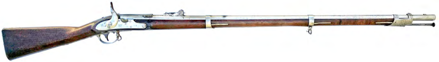
Figure 2. The Morse alteration of a Model 1866/22 .69 caliber musket retains the original length of the barrel/breech system of 42 inches, but the in-the-bore barrel length is now 38 inches. The production muskets were rifled and had long range rear sights added. The musket's metal parts are finished in-the-white, while the breech system also appears to have been identically finished (but here is tarnished). The walnut stock is oil finished. (Author's collection and photo)
