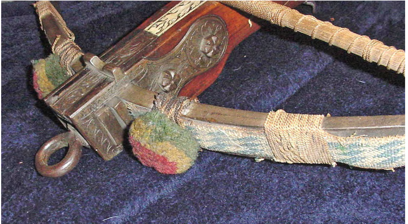
Figure 8. The fabric strip on the front of the lath serves two purposes, first the decorative colors of Bavaria, yellow and blue, but also is a safety factor to control backlash should the lath break during use.
