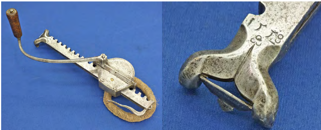
Figure 3. The cranequin was a precisely-made geared machine capable of spanning the most powerful crossbows; the date “1558” appears on the hook end. The armorer’s mark indicates that it was made in Zurich. An identical one, dated 1556, is in the Metropolitan Museum of Art Collection. Dick Salzer Collection.
