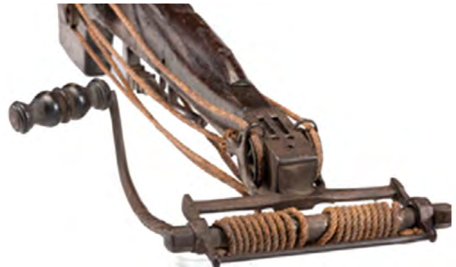
Figure 1. The windlass type spanner, shown in part, here, was detached after spanning. A single windlass was shared by several shooters.
