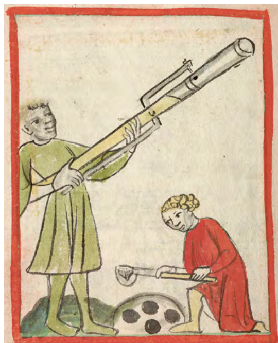
Figure 1. A simple serpentine gun, 1411. Austrian National Library, Vienna, Codex Vindobana 3069, f. 38v. A crude barrel is pole-mounted and fired with a Z-shaped metal arm (serpentine). The other figure is casting bullets.
