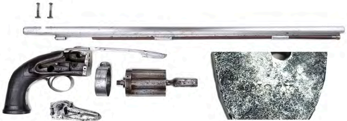
Figure 24. Collier First Model rifle No. 6, with clockwork action. Even though in 'dug-up' condition, it reveals "S. Nock" as the lock maker, and the presence of the spring that powered the cylinder rotation (Institute for Military Technology).
