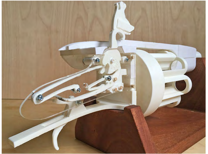
Figure 25. Digital drawing and model of ‘Collier No.7’ pistol, using a 3D printer, laser-cut acrylic and sundry items from the local hardware store (Danny Salomoun, Chris Andras, Alejandro Finol, and Thomas Rushton).
