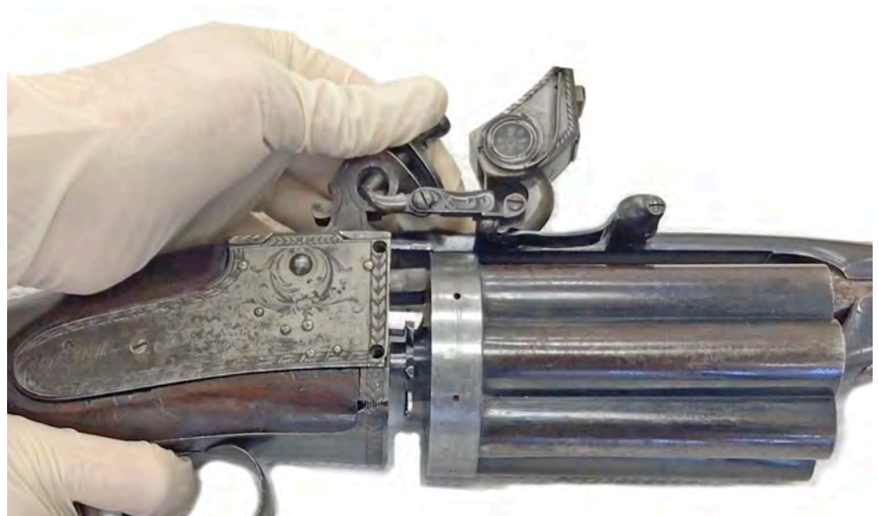
Figure 9. Collier First Model No. 5 lock with catchbolt mechanism hooking onto the ratchet wheel on the rear of the cylinder. (source: Nebraska History Museum; object ID 8241-252).
