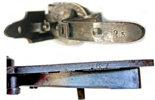
Figure 18. Four examples of 'serial' numbers stamped on the seven assemblies of the Second Model Collier (sources: top - Frank Graves Collection; middle two images - Peter Baldwin Collection, U.K.; second from bottom - Auckland Museum W0100 38005.63; bottom - Victoria & Albert Museum M.680-1927).
