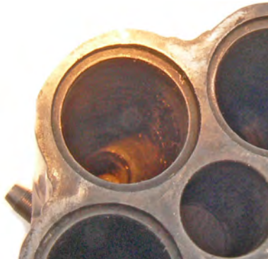
Figure 22. A Collier Third Model cap lock pistol No. 106, showing the necked-down cylinder and an opening cut in the upper rib (top strap) to permit the nipples to pass. At the base of each chamber (No. 192) is a narrow tunnel (source: location not known, photographs by Frank Graves).
