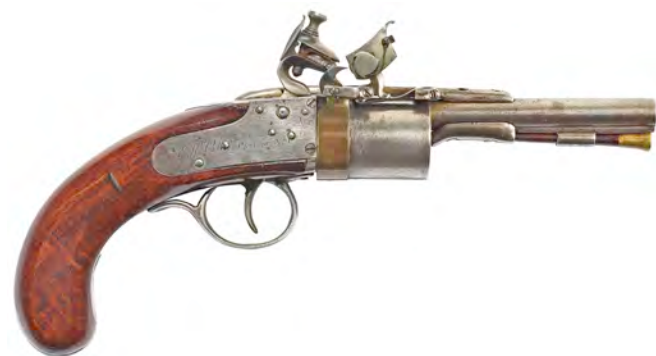
Figure 5. Collier First Model No. 1, flintlock pistol, manually rotated 5-shot cylinder, fitted with a multi-charge magazine frizzen (source: National Museum of American History (NMAH) ID number AF.81317M).
