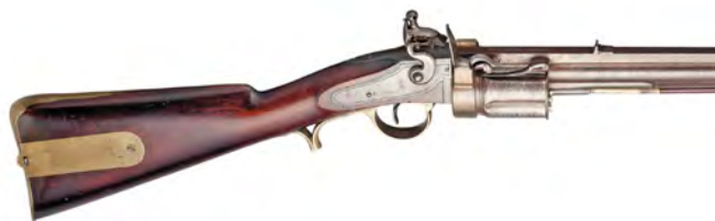
Figure 10. Collier First Model, un-numbered (# F-C), flintlock 5-shot manually rotated cylinder with a scrape primer magazine. This version was modeled after the Baker rifle (source: Christie's, 2013, lot 96.).
