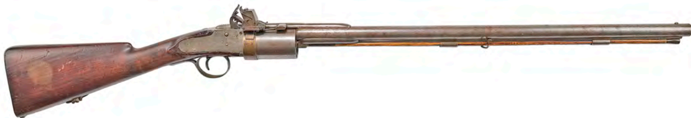
Figure 11. Collier No. 17 is a manually operated five-shot rifle. Its assembly number is "5", internal scribed letters are "VIII", in addition to the lockplate number "17". This may indicate that it was the fifth prototype that Collier built (source: NMAH; ID number AF.85467M).
