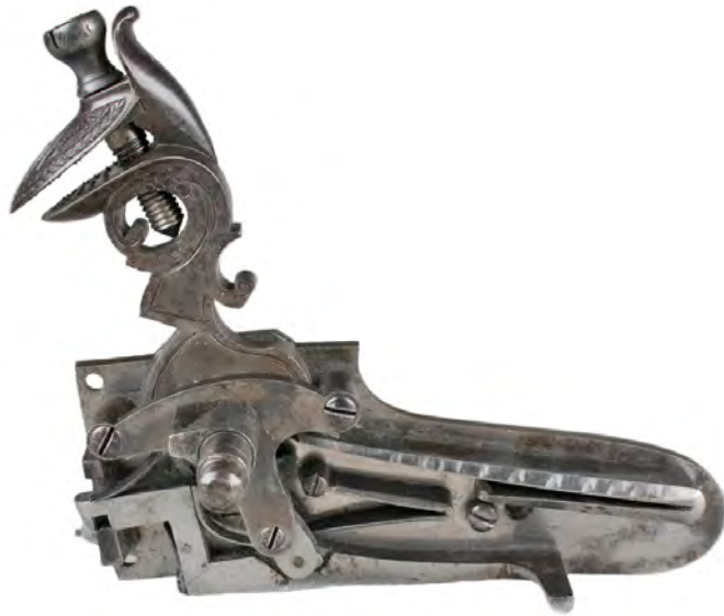
Figure 8. Collier First Model No. 5 lock with catchbolt mechanism (source: Nebraska History Museum; object ID 8241-252).
