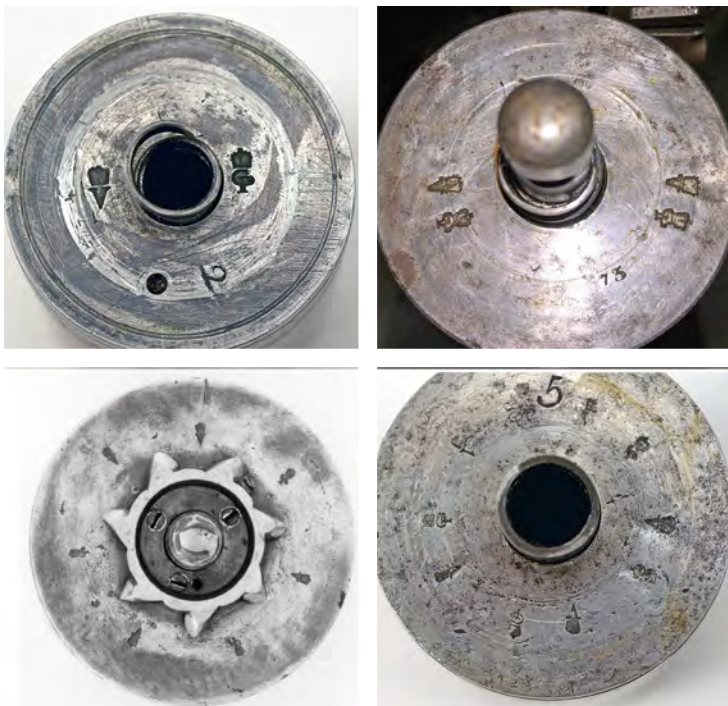
Figure 17. Four different systems of proving the cylinders of Collier revolvers. Top left, clockwise - One pair of V & GP, No. 1 (sources: top - N.M.A.H. AF.81317); Two pairs of V & GP, No. 125 (No. 73; Museum of Connecticut History TG 67); Five pairs of V & GP, No. 17 ( NMAH AF.85467M); Alternating V or GP, No. 4 (Royal Armouries XII.1503).
