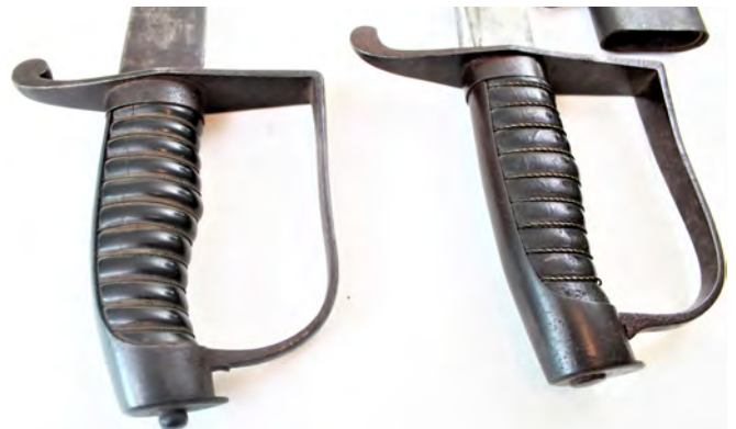
Figure 8. Here is a comparison of the Rose ebony grip from a commercially made and sold Rose saber on the left and an 1807 contract saber with leather covered grip on the right. Also note that the left grip has a capstan while the 1807 contract saber, the one on the right, has a button. The War Department sabers did not have capstans, most had a button while others were smooth peened possibly from later tightening efforts. Nothing in the government documents indicate the button affectation. The pommel cap top is a separate piece of steel braised on and has a small lip on the underside toward the stirrup or "D" shaped knuckle bow. (Rose on the left courtesy Dave Terefenko and on the right Author's collection)
