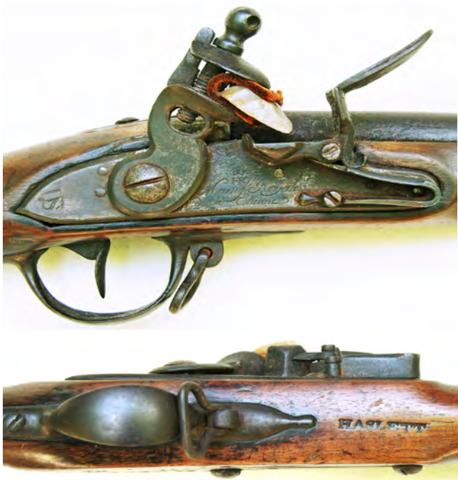
Figure 15. Lock (top) and Haslett’s mark on the repaired musket in the display (bottom).
