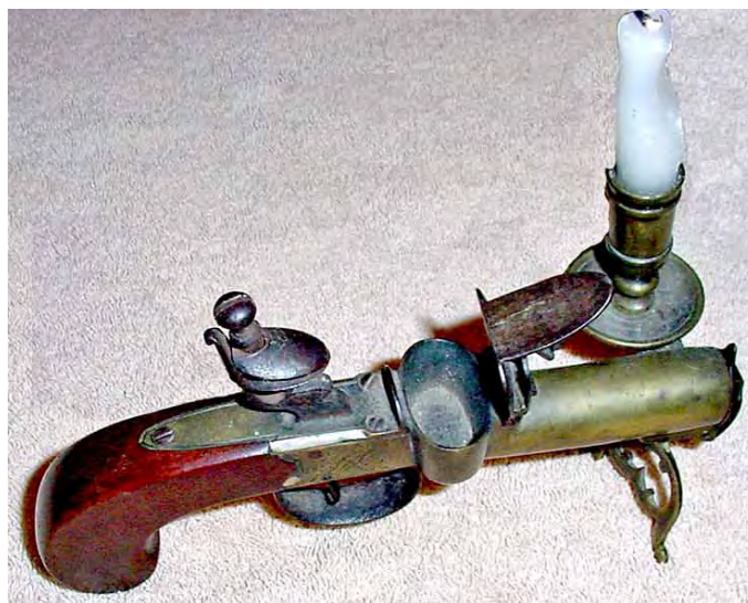
Figure 6. An unusual pattern of tinder lighter. The “barrel” is actually a tinder storage compartment and has a spring-loaded door closes of the storage chamber.
