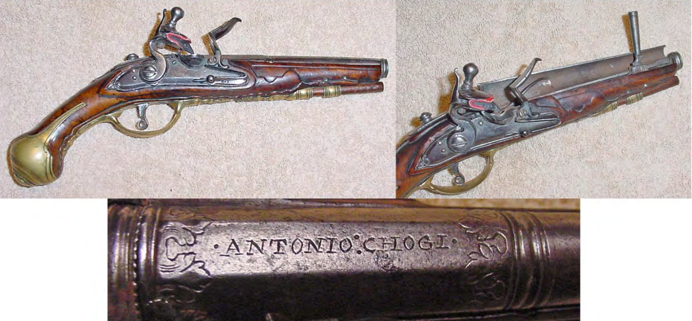
Figure 14. Italian gun maker Chogi made up a few tinder lighters based on his pistol design. On the left, it would seem, at first glance, to be a normal pistol but pulling the trigger deploys a lighted wick, as shown on the right. Full page width
