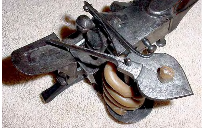
Figure 10. A most unusual design, incorporating a scissor to snip off a length of candle from the coil.
