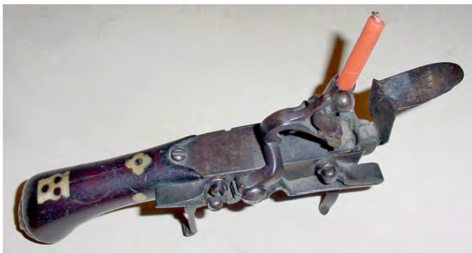
Figure 3. A nice little, well-made lighter decorated with bone inlays. Like most lighters, it contains a compartment for storage of tinder.
