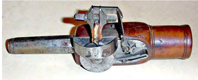
Figure 8. Possibly the only known Wheellock lighter. Activated by a pullcord attached to the wheel.
