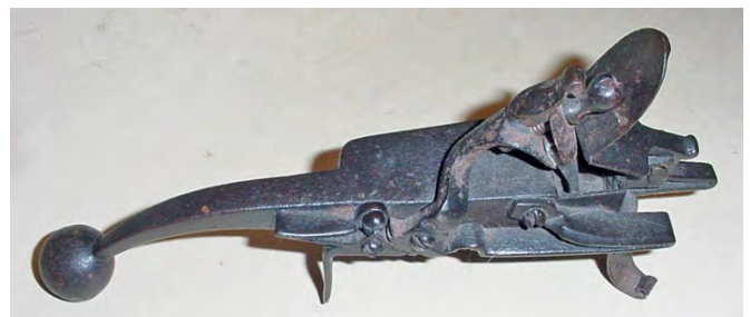
Figure 1. This form is generally called “rat tail”, this one is iron but the pattern is more often found in brass.
