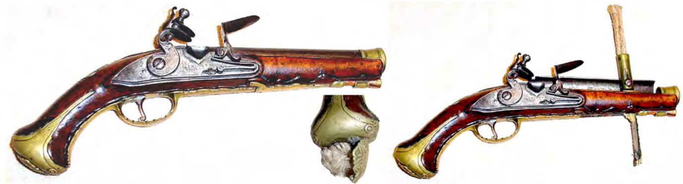
Figure 13. A few gunsmiths took delight in creating pistols that were actually tinder lighters. Like the specimens shown, they give every appearance of being a regular pistol. When the trigger is pulled, the lock fires and the lit wick pops up while the stand deploys downward (right panel). A few grains of black powder insures ignition. The buttcap is hinged, revealing storage for extra tow (inset).
