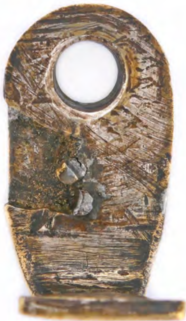
Figure 9. Cocking the pistol. Curved slot on the interior bottom of the trigger guard positions the trigger lever.
