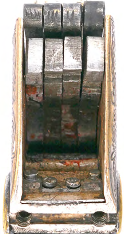
FOUR FIRING PINS, FOUR COCKED HAMMERS, AND FOUR MAINSPRINGS WITH SLASH MARKINGS
