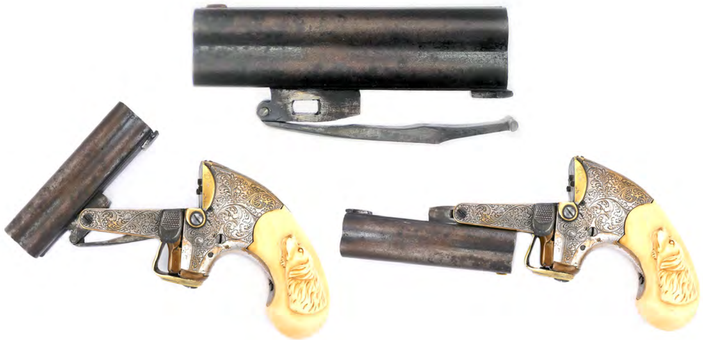
Figure 11. Cocking the pistol by tilting the barrel. Clockwise from top: barrel block with tenon, oblong slot, and cocking arm with a T-bar end within the frame which presses against the hammers; With the trigger guard positioned slightly toward the right over the trigger, depressing the barrel-release slide and lifting the barrels to a 45-degree angle begins the rearward motion of the cocking arm; After pulling the barrels upward, the barrels can continue in a 180-degree arc, moving the cocking arm rearward into the frame and fully cocking the four hammers.
