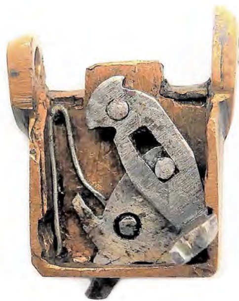
Figure 10. Cocking the pistol. Interior of the box trigger showing the spring-loaded trigger lever (protruding from bottom) which controls the vibrating trigger arm (right).
