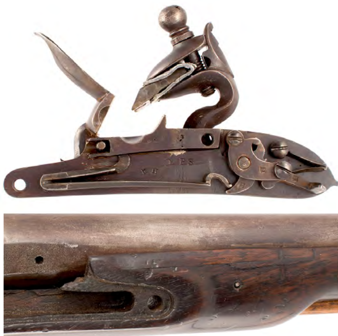
Figure 32. Interior of lock plate from Henry Repeater pistol that was modified for the Chambers system (top). Note the portion of the lock where the frizzen screw is located that was milled out to accommodate the priming tube. The image below shows the spline of wood that was added to replace the space where the priming tube was.
