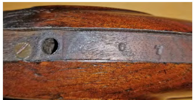
Figure 9. Tang mortise, note the assembly number “7” stamp on the right side of the mortise.
