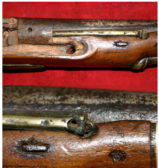
Figure 29. Harpers Ferry Pistol barrel with Chambers tube and close up of clean out door (bottom)
