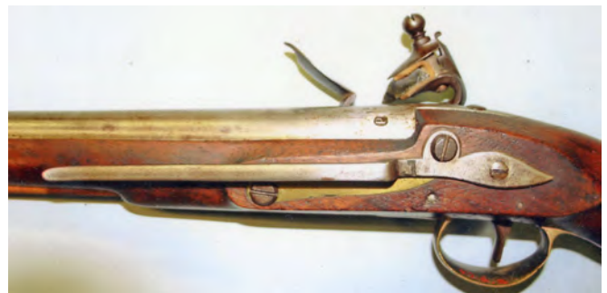
Figure 27. Belt hook on Perry Navy pistol.
