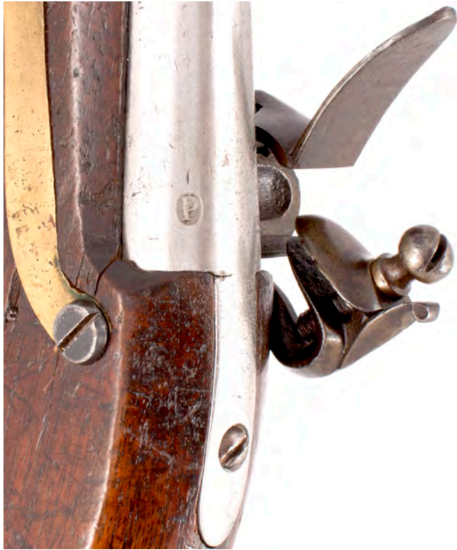
Figure 37. Henry barrel proof on the “Better Kind” of pistol.
