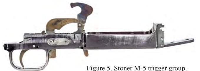
Figure 5. Stoner M-5 trigger group.
