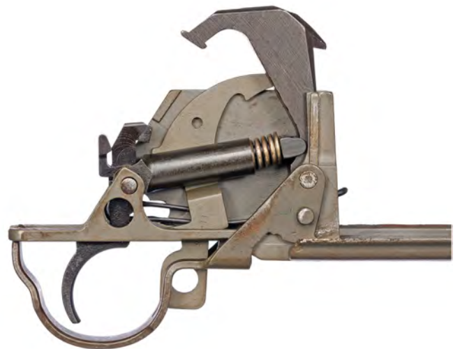
Figure 6. Trigger mechanism for a Johnson 1941 rifle (left) and M1 Garand trigger group (right).
