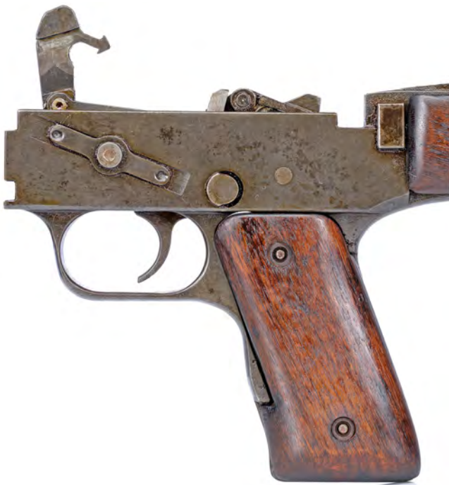
Figure 6. Trigger mechanism for a Johnson 1941 rifle (left) and M1 Garand trigger group (right).
