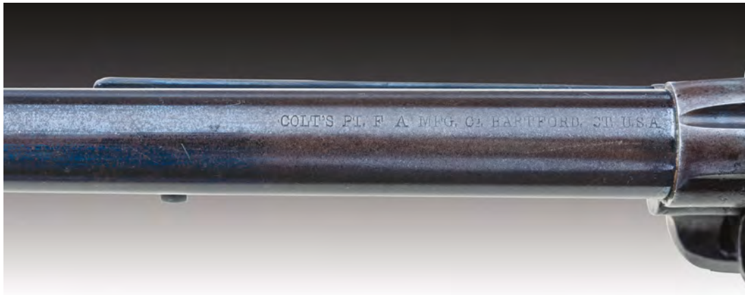
Figure 4. Block style barrel address for Colt Single Action Army revolver, serial number 40956, caliber .44-40 WCF.
