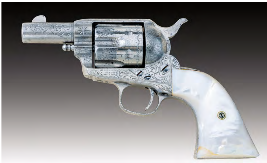
Figure 11. Colt Frontier Six Shooter Sheriff's model, serial number 115126. .44-40 caliber, 2 1/2" barrel, ejectorless. Nickel finish, pearl grips and factory engraved. Shipped February 3, 1886 to A. G. Spaulding Brothers, Chicago, Illinois. One of one manufactured. NRA silver medal 2018. 9
