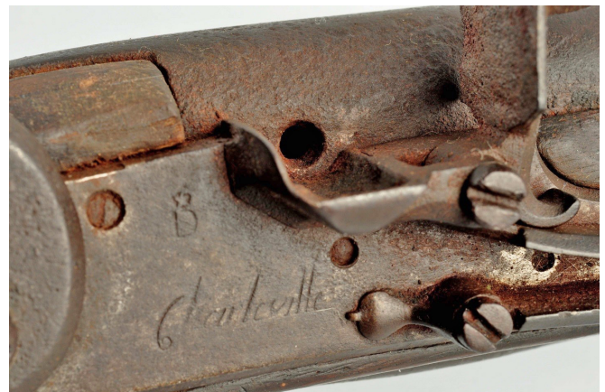
Figure 3. Touchhole of the French Model 1766 Charleville musket believed to be modified with “Wayne’s improvement”.
