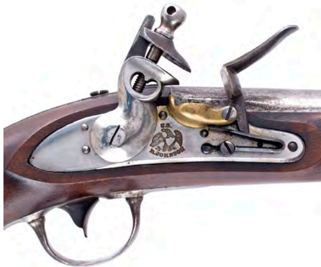
Figure 2. Close up of the lack plate for the Pattern Pistol of 1840, note the eagle stamping with "R. Johnson" in an arch below.
