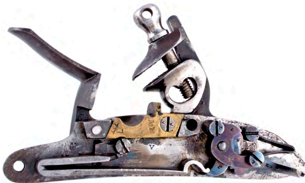
Figure 3. Lock plate interior of the Pattern Pistol of 1840.
