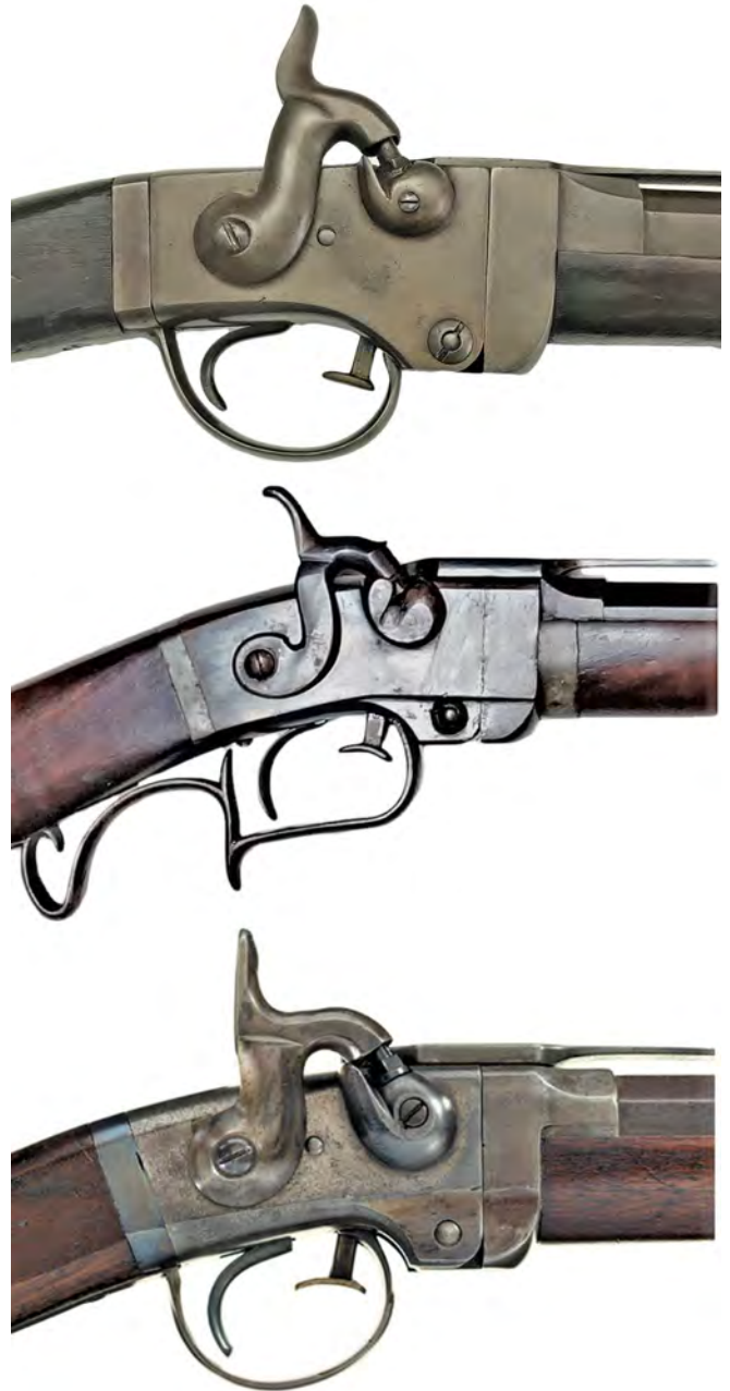
Figure 1 Progression of Smith receiver design; top early military carbine; middle commercial "sportsman" carbine; bottom CW Production carbine (Authors collection).
