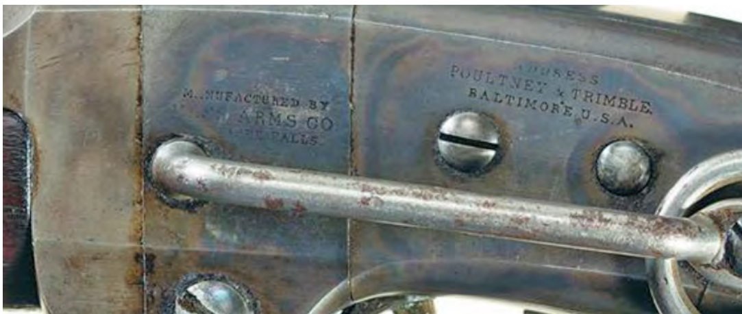
Figure 20. Receiver markings on Smith carbine, serial number 14392, manufactured by Massachusetts Arms Company. The Smith patent markings are obscured by the sling bar (Photograph courtesy of Rock Island Auction Company).
