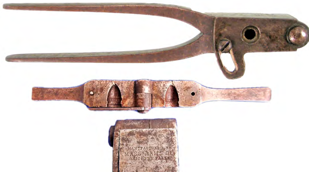
Figure 13. Single cavity bullet mold manufactured by Massachusetts Arms Company for Model 1861 Smith Carbines (Don Dietrich collection).
