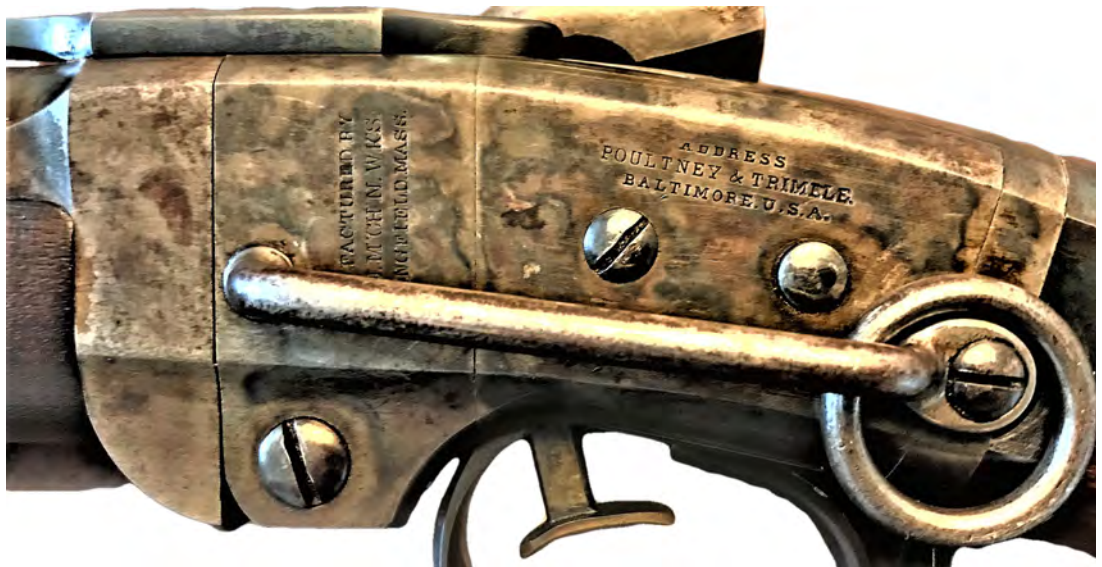
Figure 22. Receiver markings on Smith carbine serial number 3454 manufactured by the American Machine Works. Smith Patent marking is obscured by the sling bar. (Author's collection).
