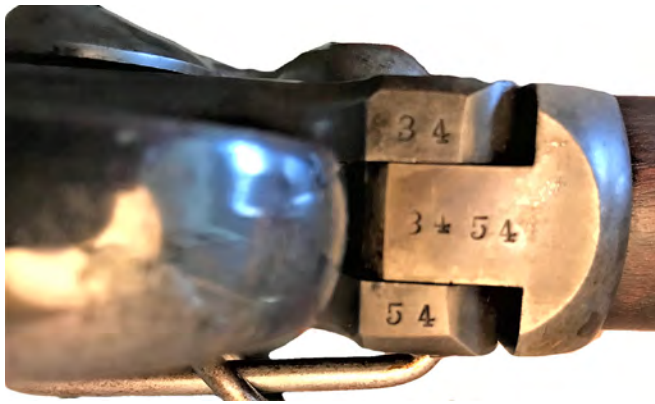
Figure 24. Placement of serial numbers on Model 1863 Smith carbines (Author's collection).
