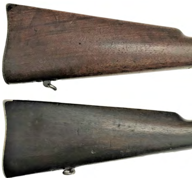
Figure 3 Comparison of the location of the rear sling swivels; top shows placement on the Civil War production Model 1861 carbine and bottom shows placement on early Model 1859 military carbine (Authors collection).
