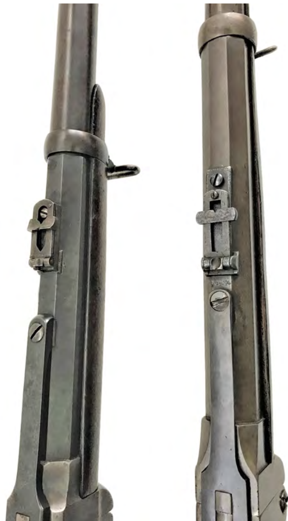
Figure 4 Comparison of rear sight on military carbines. The Civil War production carbine Model 1861 sight is shown on the left and the Lawrence patent rear sight mounted on the early Model 1859 military carbines is on the right (Authors collection).
