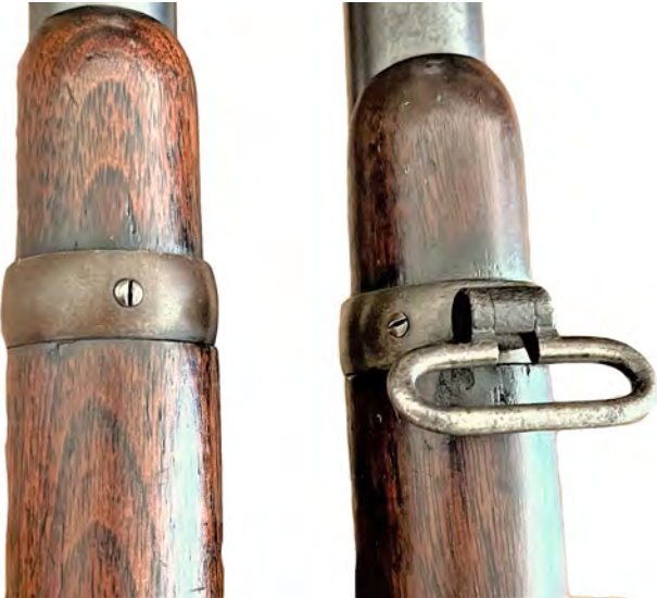
Figure 17. Barrel bands on Model 1861 and Model 1863 carbines showing offset band retaining screw on the earlier carbine (left) and central position of the screw on the later (right, Author's collection)
