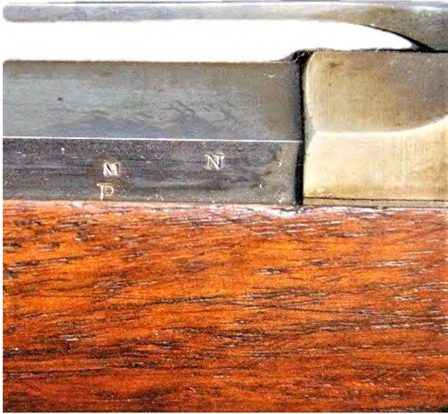
Figure 30. Barrel proof stampings on Mass Arms Co Smith carbine serial number 19596 (Photograph courtesy of Rock Island Auction Company).
