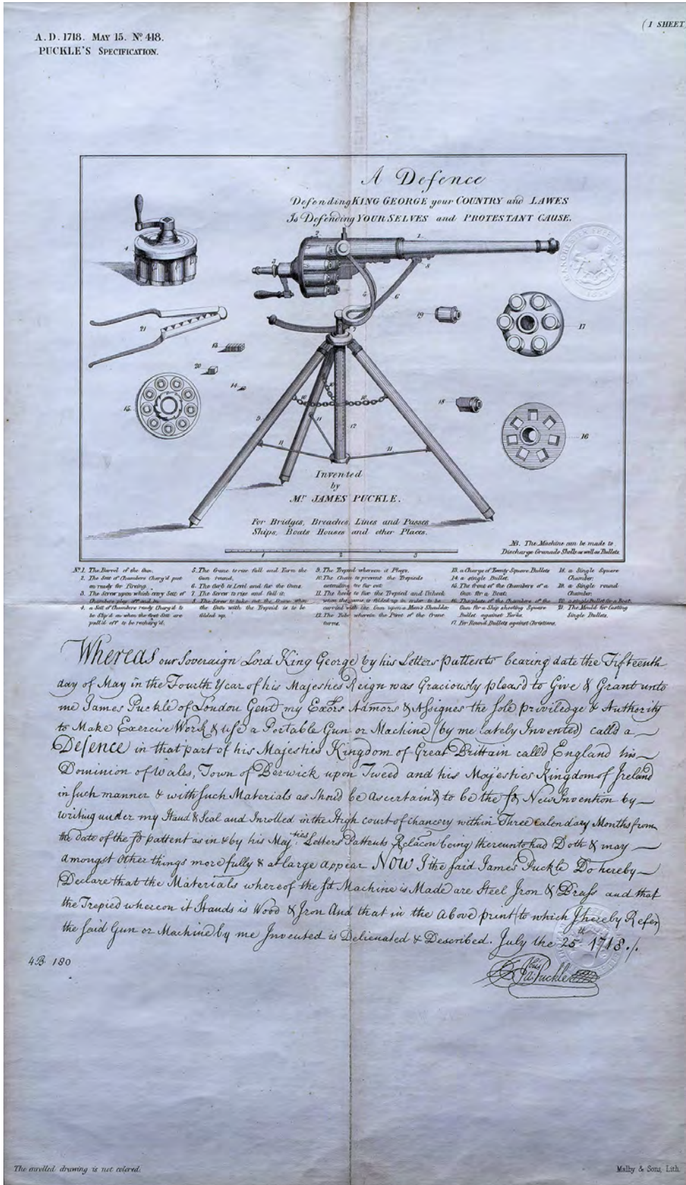
Figure 1. Original patent for the Puckle gun.
