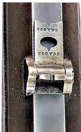
Figure 5. Single leaf rear sight mounted on Ballard military firearms (Author's collection).
