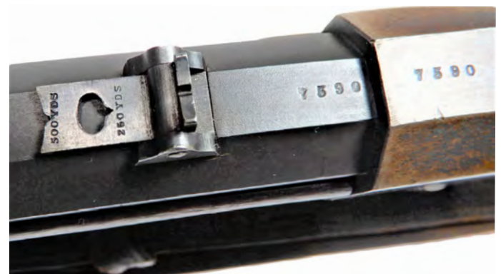
Figure 7. Rear sight on Model 1862 rifle, serial number 7590 (Author's collection).
