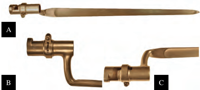
Figure 22. The Model 1851 Cadet bayonet (A). Note the unique lockup arrangement, with two shoulders and a slotted locking ring (B, C). The standard "US" marking is found on the blade face. The number "49" appearing on both the locking ring and the socket are thought to be of Virginia Military Institute provenance (A and C). A number stamped at the base of the socket, "224" in this example, is consistent with other bayonets of this type, although of unknown origin (B).
