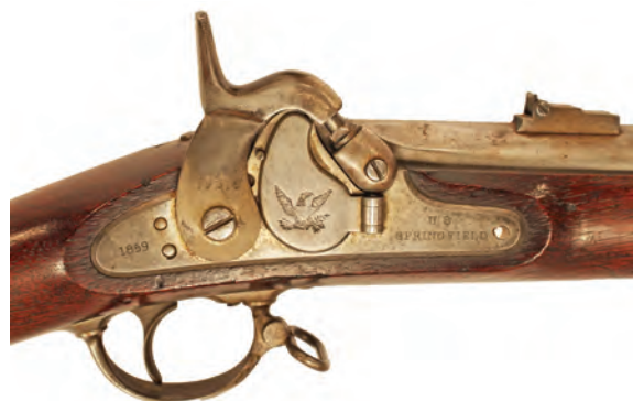
Figure 24. The Model 1858 Cadet Musket retains most of the components of its parent Model 1855, including the lock system with the innovative Maynard tape priming feature.
