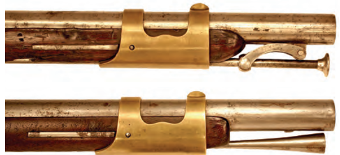
Figure 17. Muzzle-end comparison of original Cavalry Model (top) and Cavalry Model with Artillery/ Cadet alteration (bottom). In this alteration the brass furniture was retained throughout. Note the addition of a bayonet lug in the bottom photo.
