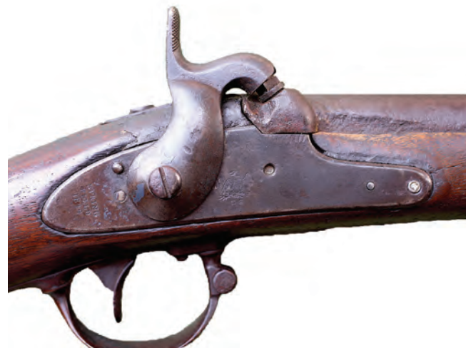
Figure 14. The lock design for the 1841 Cadet was borrowed from the Harpers Ferry Model 1841 Rifle.
