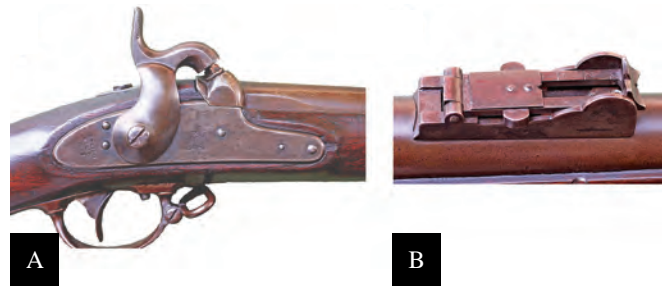
Figure 21. The Model 1851 Cadet lock is the same as what was used in the 1847 Musketoon (A). A Model 1855 rear sight was added in 1857, along with rifling, to some 323 Model 1851 Cadet Muskets held in storage (B).
