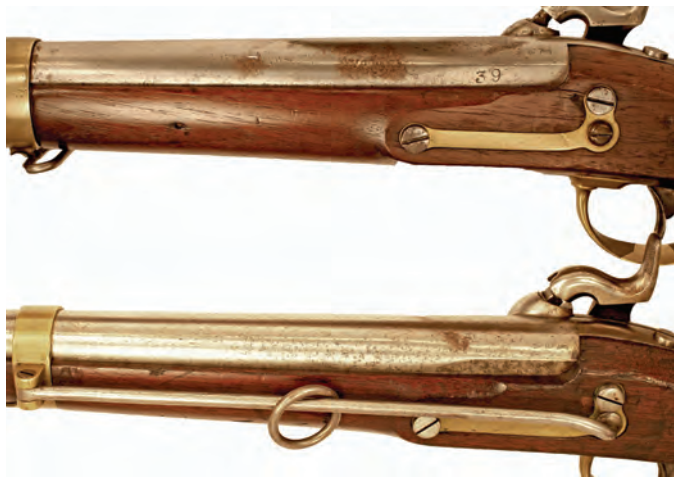
Figure 18. Comparison between the original Cavalry Model (bottom) and Cavalry Model with Artillery/ Cadet alteration (top). In the top photo, note how the barrel band was salvaged by removing the sling bar lug and adding the sling swivel lug.
