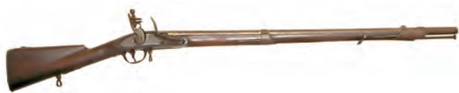
Figure 3. A Charleville Pattern musket that was originally equipped with a soldered-on bayonet and subsequently cut down to 33 inches in the 1813 alteration program at Springfield Armory. Note the “Brown Bess” method of upper sling swivel attachment. These were thought to be among the first of the reduced-size guns that went to West Point.
