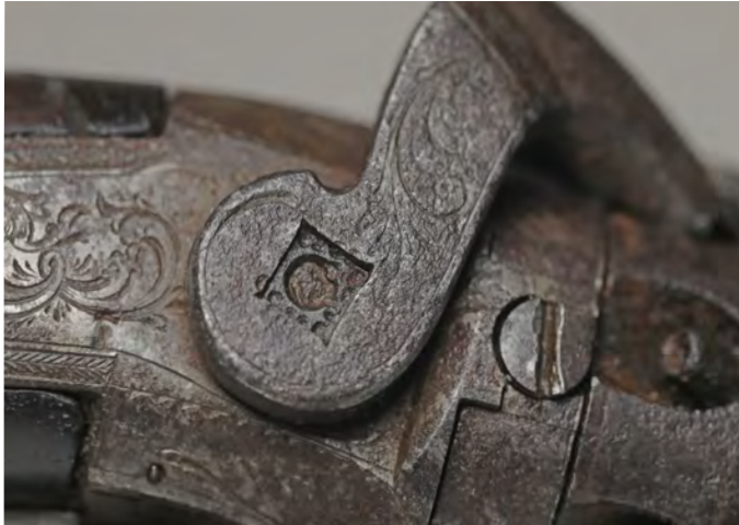
Figure 9. Attachment of the hammer on the New Haven bar gun. Photo by Don Summers.
