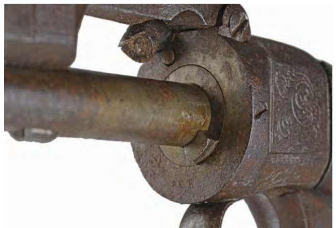
Figure 3. Breech face showing "sleeve or collar" protrusion on the New Haven bar revolver. Photo by Don Summers
